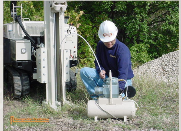
The Portable Vacuum Volume System is easily transported to the field for use with Soil Vapor Implants or Geoprobe® PRT System.
