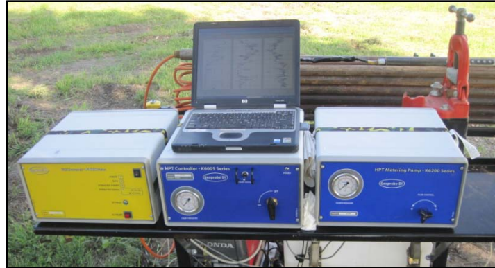
Figure 7: The HPT flow controller (center) receives water from the pump (right) and regulates flow to the probe. The FI 6000 Field Instrument (left) supplies conditioned current for the EC measurement, receives analog signal from the HPT probe and provides digital output to a lap top computer (top center).
