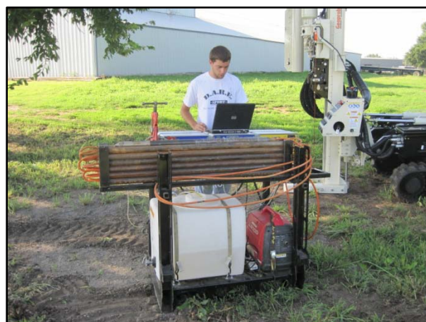
Figure 6: Probe rods are prestrung with the HPT trunkline and may be stored and transported on a Geoprobe® drop rack. In this setup the water tank, generator and instrumentation may be loaded on the rack for easy transportation on site.
