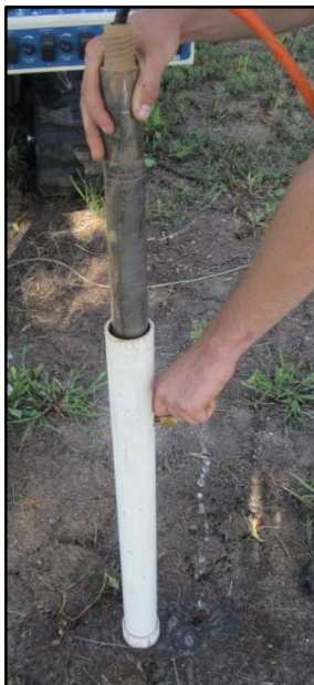
Figure 9: The HPT probe is inserted in the reference tube to verify performance of the pressure transducer as a part of the pre-log QA testing protocol. The QA test provides a pass/fail report for the transducer with a know height of water column. Reference tests are saved in the information file for each log (Appendix II).
