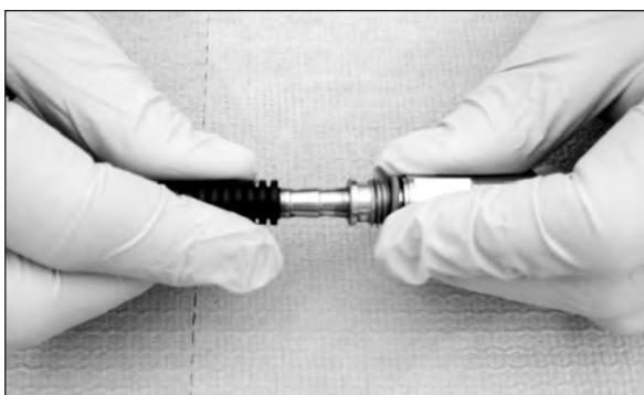
Figure 4.3: Install bladder on lower bladder adapter (PN 20677) with gentle but firm twist and push.
