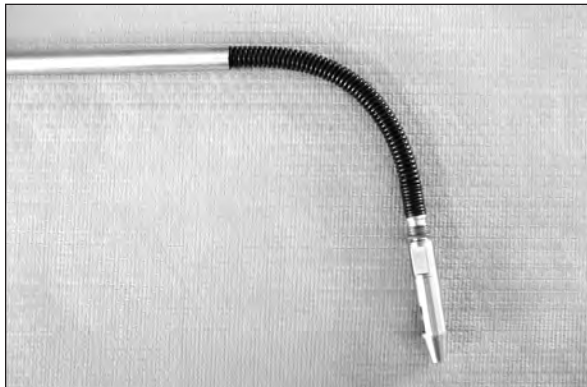
Figure 4.9: Unthread the lower bladder adapter (PN 20677) from the bottom of the pump body. This will prevent damage to the bladder as the pump body is rotated to attach to the outer tube.
