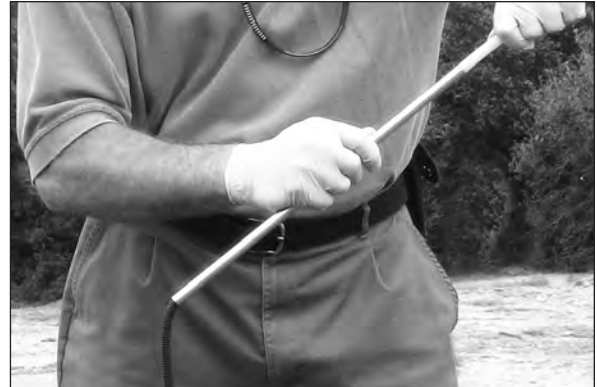
Figure 4.10: Firmly push and twist the pump body onto the outer tube. Threads inside the pump body will self-thread onto the outer poly tubing. The tubing should thread about 0.5 to 0.75 inches (12 to 18 mm) into the pump body.
