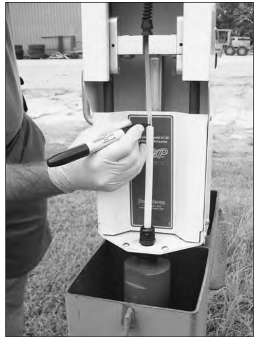
Figure 4.21: With the pump, tubing set and actuator installed on the well, be sure the slide block is at its lowest position. Now push the inner tube down firmly to compress the bladder. Mark the inner tubing at the top of the outer tubing to provide a visual reference. This mark will be used to guide the inner tube placement.
