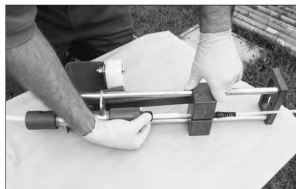
Figure 4.20: Insert the concentric tubing through both compression fittings on the actuator. Tighten the lower compression fitting to hold the outer tube in position. The outer tube should stop 2 to 4 inches (50 to 100mm) above the lower compression fitting. Do not lock the inner tube into position yet.
