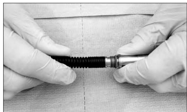
Figure 4.4: Push and twist the bladder onto the barbed fitting until 5 to 7 corrugations are compressed over the barbs. Repeat the same procedure for the upper bladder adapter (PN 20679)
