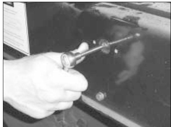
Figure 9: Reinstall the grease zirk with the ratchet, extension, and 7/16-inch socket.
