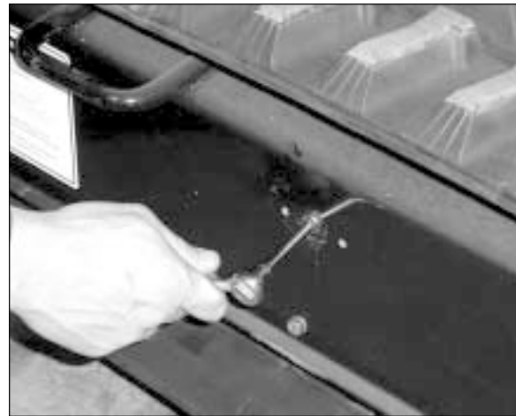
Figure 4: Remove the grease zirk from the track tensioner.
