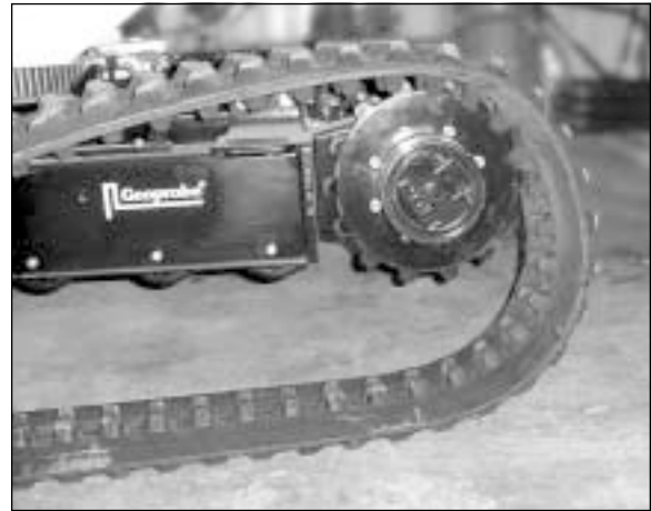
Figure 8: Place the rubber track over the drive wheel sprocket.
