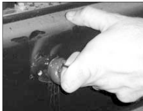
Figure 6: Grease will escape from the tube as the tension wheel is retracted to loosen the tracks.
