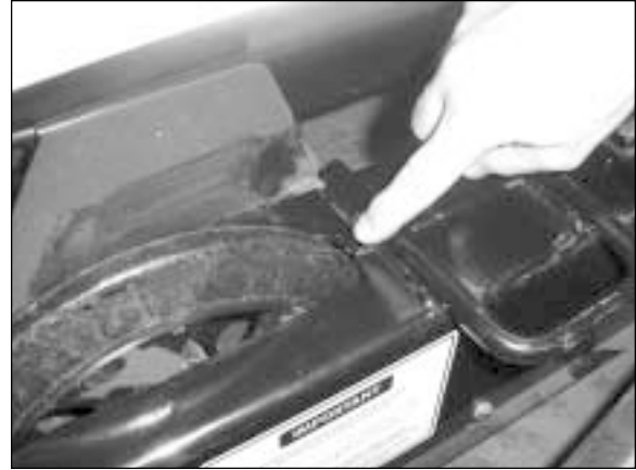
Figure 7: The tension wheel will contact the track frame when fully retracted.
