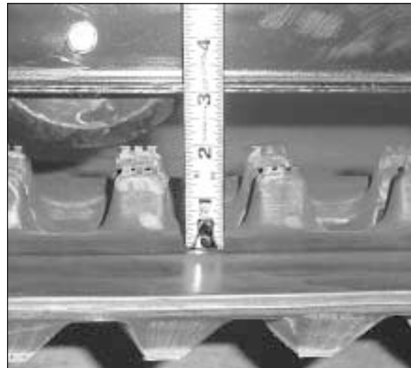
Figure 11: The rubber track should sag 2.5-3.0 inches from the center of the track frame.
