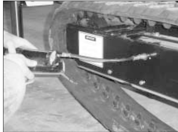
Figure 10: Pump grease into the track tensioner to tighten the rubber track.
