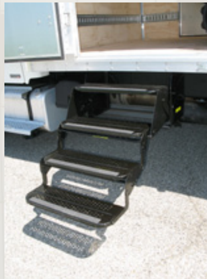
Convenient Walk-in steps are provided on the drivers & passengers side cargo doors
