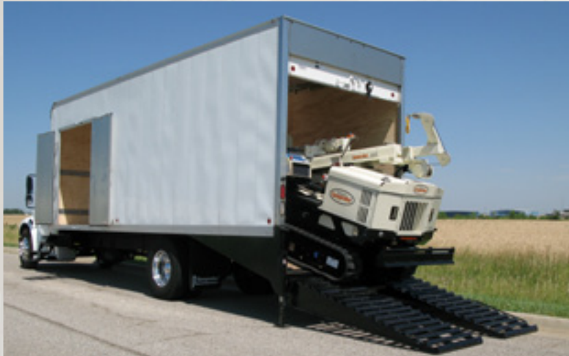
(Above) The model 7822DT machine easily loading into the transport truck using the spring assisted ramp system
