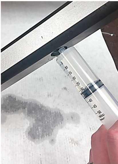
Figure 6.1: Flushing the optical cavity with water
