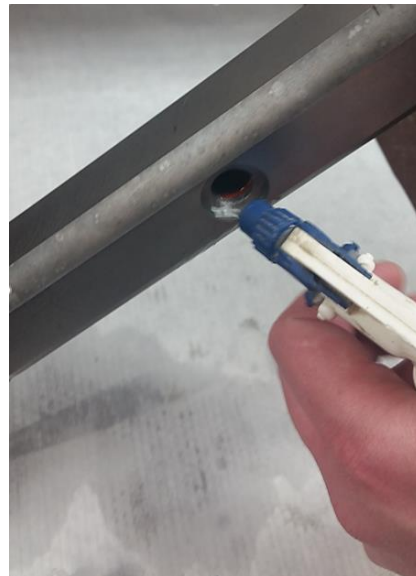
Figure 6.2: Flushing the optical cavity with alcohol
