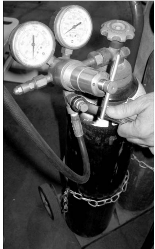
Figure 4.36: Relieve pressure from the nitrogen fill hose by slightly unthreading the bleeder valve.
