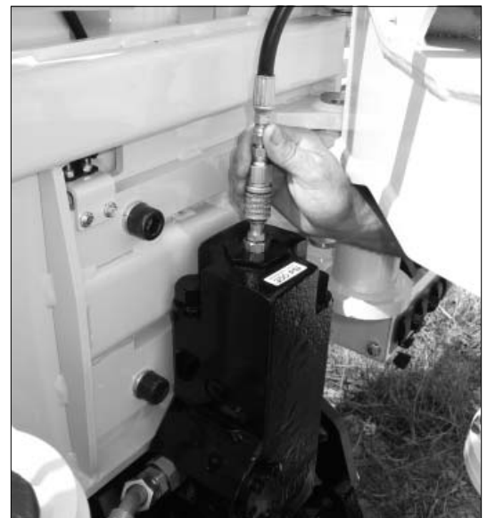
Figure 4.35: Connect the fill hose coupler to the nipple installed in the nitrogen charge valve.
