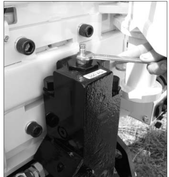
Figure 4.34: Install the nitrogen charge adapter in the charge valve assembly.
