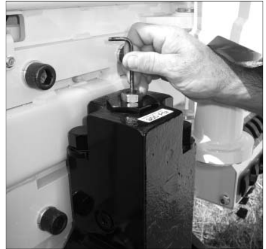
Figure 4.33: Depress the charge valve with a blunt object to discharge the accumulator.
