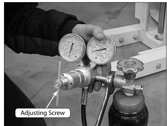
Figure 4.31: Install the regulator on the nitrogen cylinder.
