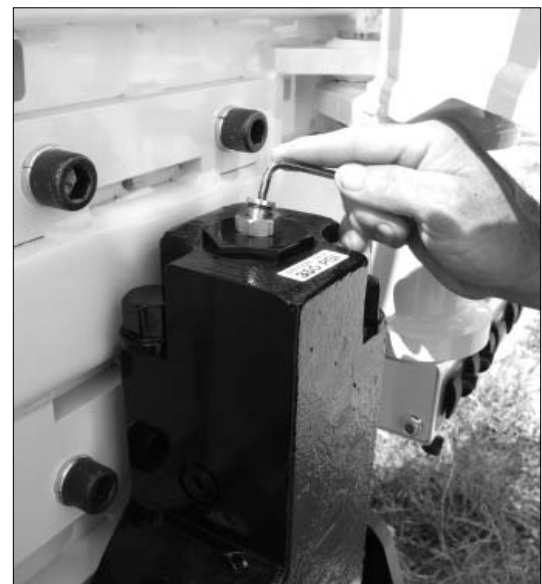
Figure 4.32: Remove the plug from the nitrogen charge valve of the TE accumulator with an Allen wrench.
