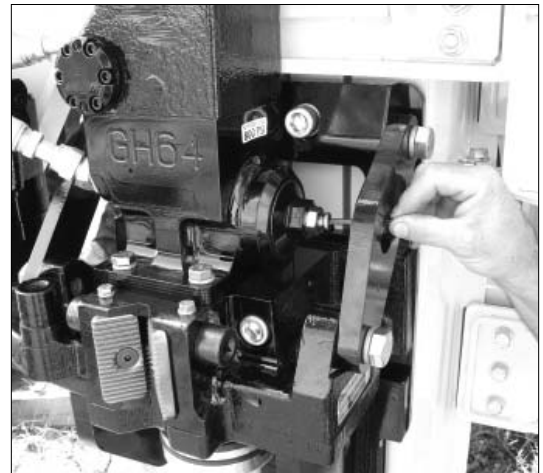
Figure 4.37: Remove the plug from the nitrogen charge valve of the SE accumulator with an Allen wrench.
