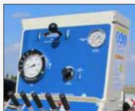
head feed pressure control module ...216137
