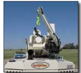
overhead mast and hydraulic winch ...215620
