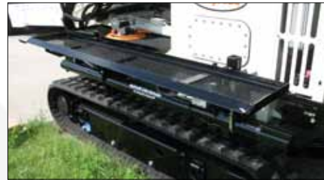
hydraulic liner extruder mount with dropdown work surface (extruder not included) ...210107
