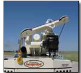
rotating overhead mast and hydraulic winch ...215728
