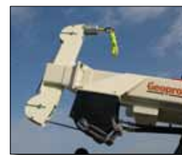
overhead mast and hydraulic winch ... 215620
