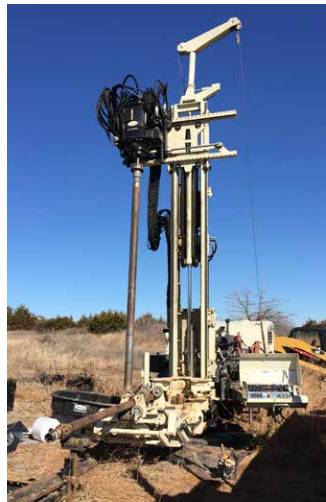
An 8150LS Rotary Sonic, owned by Associated Environmental Industries in Norman, OK, is running SDT60 and a 6.0-in. Weighted Wireline system.
