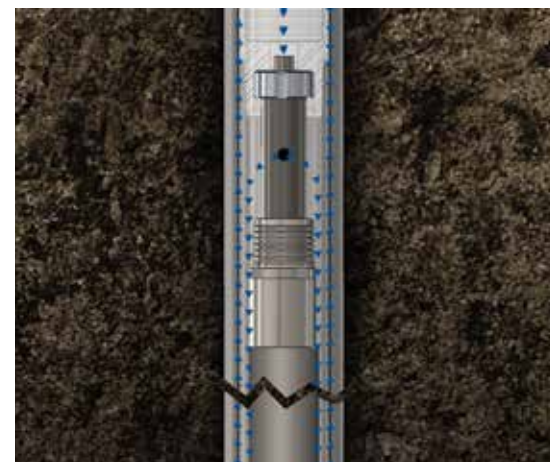
The SDW45 sonic system allows water to flow around the sampler sheath.
