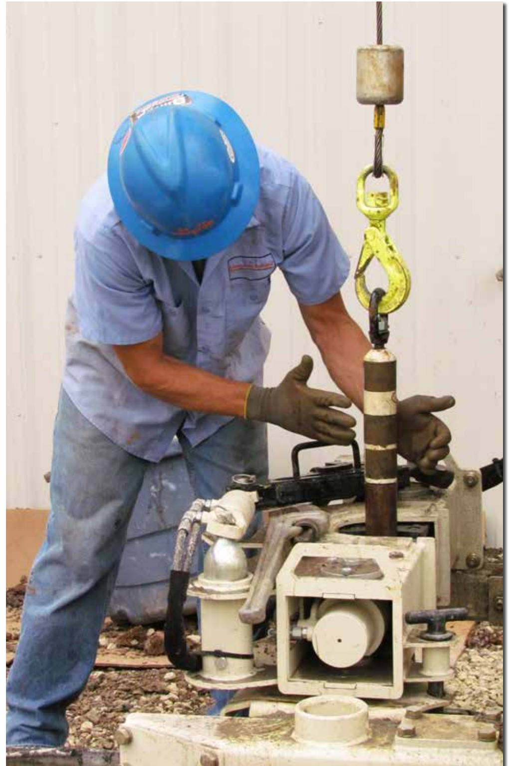
Today's larger machines enable operators to handle long sections of inner rods with an overhead winch. The 2.25-in. Spring Assisted Swivel Pull Cap is designed to reduce operator fatigue when adding or removing these sections of rods to the inner tool string ... safely and easily. Above, Lee Shaw uses the Spring Assisted Swivel Pull Cap under a 3230DT during well installation. Tooling systems that benefit from this accessory include Sonic SDT45 and SDT60, and Direct Push DT45 and DT60. Geotechnical applications include driving casing with 2.25-in. center rods and split spoon sampling with 2.25-in. rods.
