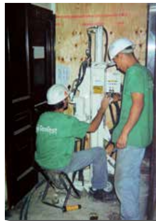
Ray Meinhardt (right) and Bill Seymour set up the GeoTest 54LT for shallow sampling work inside an office building. At 34.5-in. wide, the 54LT fits through most doorways.
