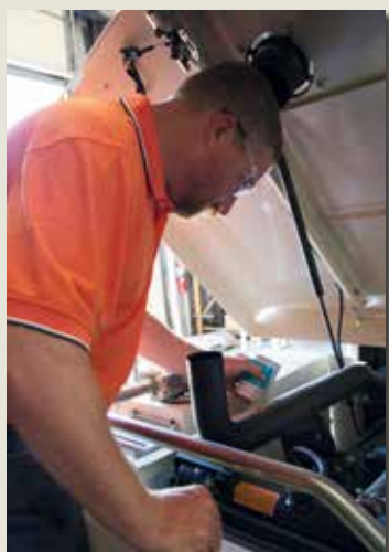
Regular fuel system maintenance is important for a happy machine. Remember: NEVER pre-fill a fuel filter for your Geoprobe® rig, and ALWAYS fill your rig's fuel tank at the end of the day.
