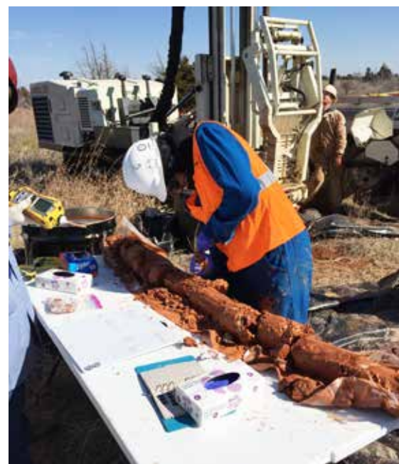
Sonic soil cores are examined in the field by an onsite geologist. The cores were retrieved by running SDT60 and an 8150LS.
