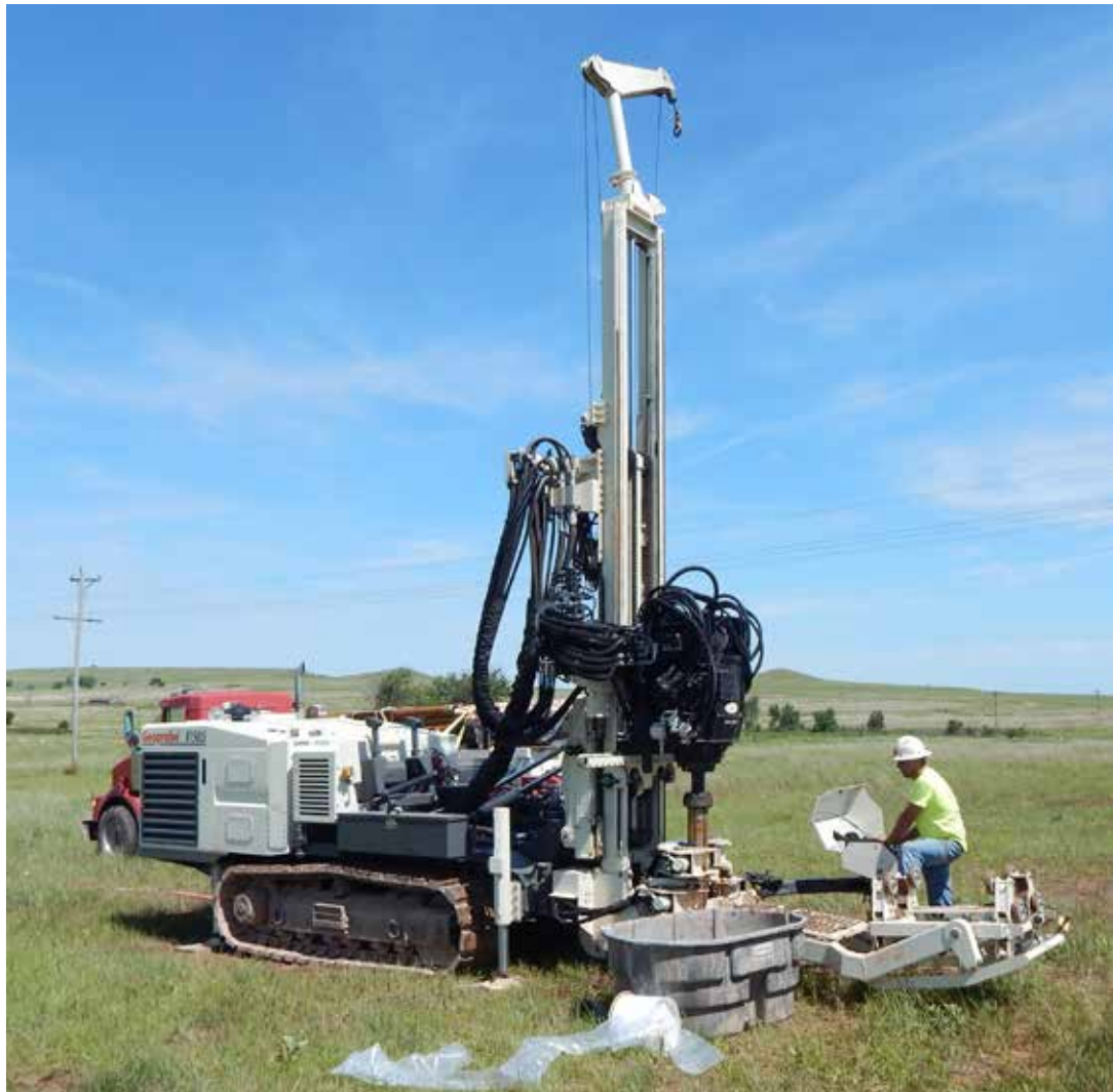
A man and his machine. Billy Graham, AEI Senior Environmental Driller, drills in the red dirt of central Oklahoma with AEI's 8150LS Rotary Sonic.
