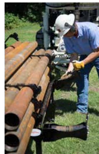
The indexing rack has two, 12-in. rubber rollers that do all the heavy lifting during trip-in and trip-out operations. The rollers feature a unique latch arrangement so they can be easily positioned up and down for each row of tooling being used.
