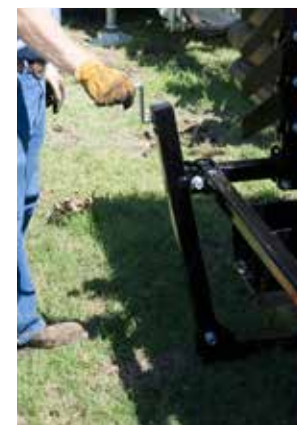
The rack also utilizes two, adjustable, mechanical jacks so the height and approach angle to the loader can be adjusted for uneven ground.
