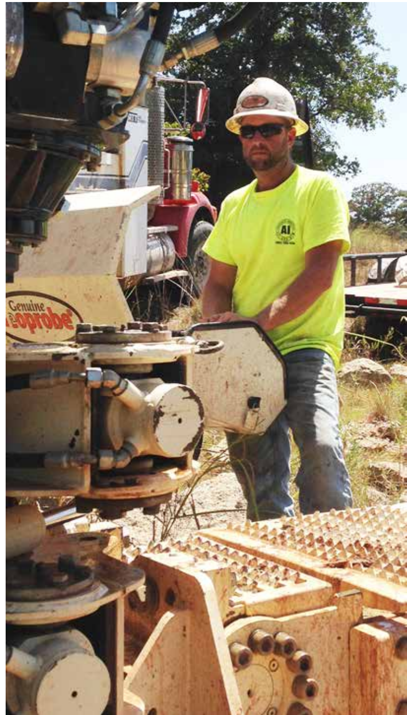
Billy Graham, Senior Environmental Driller with AEI in Norman, OK, runs 'his' sonic rig, a Geoprobe® 8150LS.
