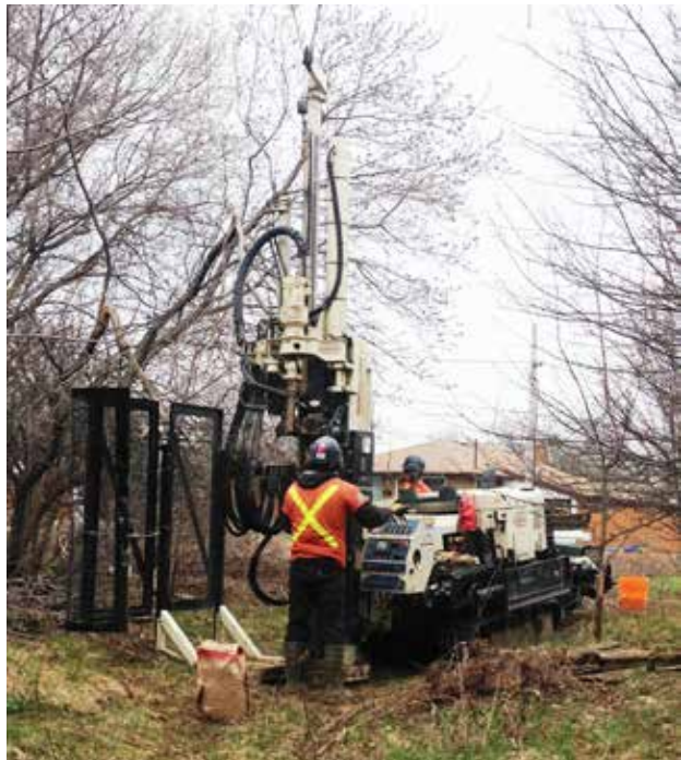
CJ, Driller, and Dalles, Helper, collect MC5 samples with a 7822DT in Cambridge, Ontario.
