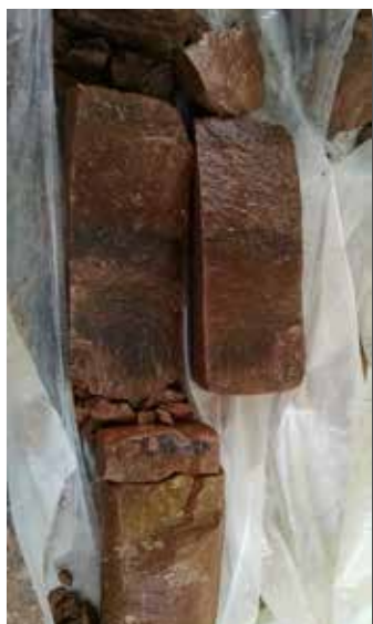
Rock core recovered using SDT60 Weighted Wireline Tooling.
