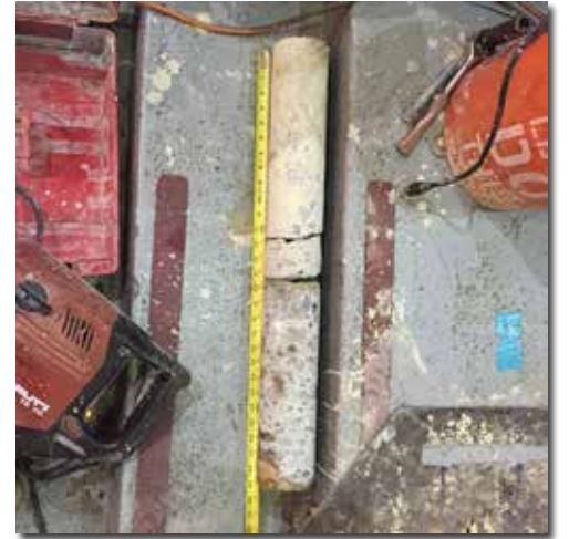
GeoTest Services collected approximately 30-in. long concrete cores with a 420M as part of the project for five limited access borings at the University of Houston inside the main auditorium of the Hofheinz Pavilion. The concrete coring was through hard rock aggregate concrete found in the older structures in Houston.
