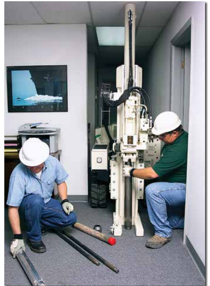
Ray Meinhardt (right) and Bill Seymour set up the GeoTest 54LT for shallow sampling work inside an office building. At 34.5-in. wide, the 54LT fits through most doorways.
