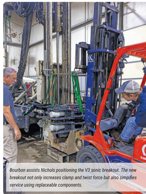
Bryce Nichols, service technician and former machine design engineer, refers to documentation while preparing to install the V3 sonic breakout on the legacy 8150LS sonic rig.
