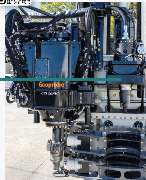
Geoprobe® engineered and manufactured GV5 sonic head with DMR7 rotary head along centerline head side shift to position over hole without moving machine.
