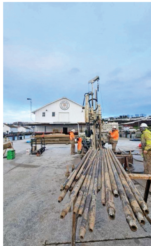
7822DT sets 4.25 hollow stem augers off the end of a dock on Mackinac Island. They performed mud rotary out the end and pulled the rods before taking a split spoon sample. In search of bedrock, they sampled every 5 feet.
