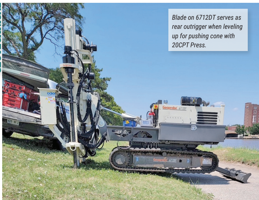
Small footprint permits 6712DT to access tight urban locations for shallow logging and soil investigation.
