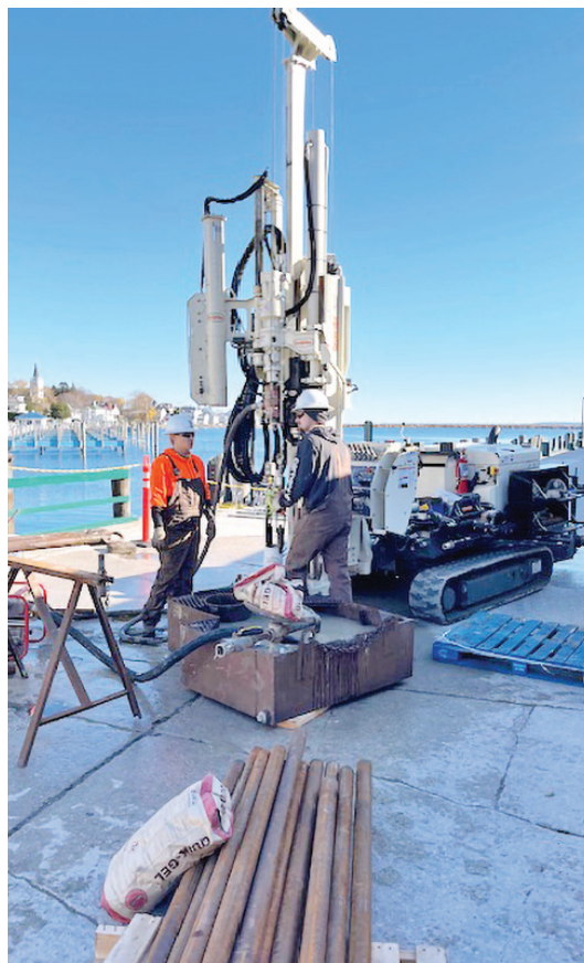
7822DT sets 4.25 hollow stem augers off the end of a dock on Mackinac Island. They performed mud rotary out the end and pulled the rods before taking a split spoon sample. In search of bedrock, they sampled every 5 feet.
