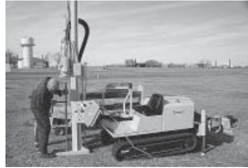
Geoprobe Model 54DT was used to advance the SC310 Expendable Dipole Probe over 80-feet below grade. The 12-volt outlet (Power Point) on the 54DT and a power inverter supplied all of the power required to operate the E-log hardware and computer.
