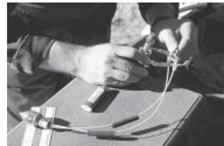
Attaching the SC310 Probe to the signal cable using heat shrink tape and micro-torch. A heat gun can be used on the shrink tape.
