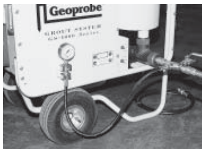
Closeup of the GS1000 Grout Machine showing the in-line pressure gauge and relief valve assembly (GS1090) used to monitor injection pressure of the 25% solids bentonite slurry.
