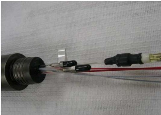
Fig. 12: Heat shrink around thermocouple connection
