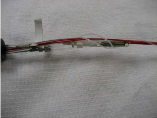
Fig. 5: Wrapping excess gas line around wires
