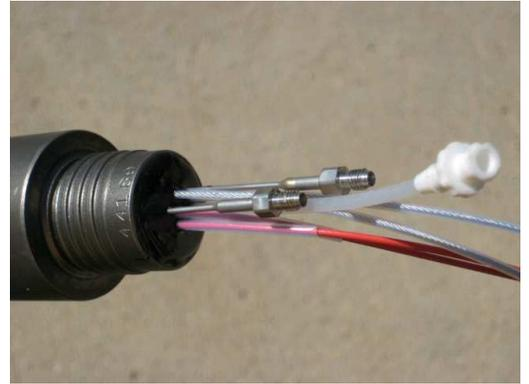
Fig. 9: Gas lines and thermocouple duct
