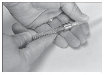
Attaching polyethylene tubing to the sampling implant.
