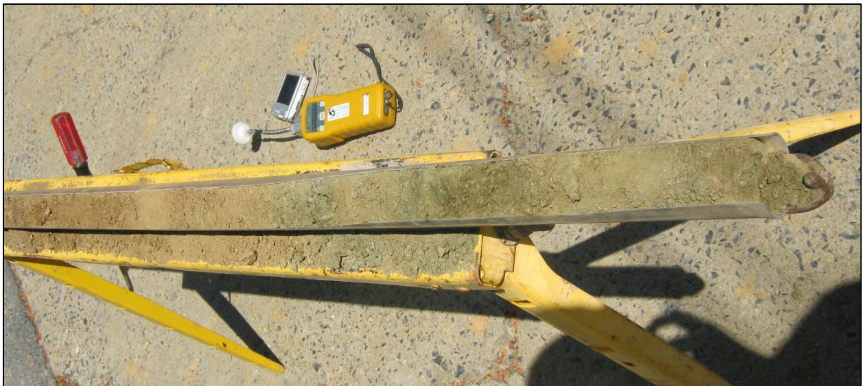
Figure 3.6. Sample of weathered bedrock showing relict fractures and discrete stained layers.
