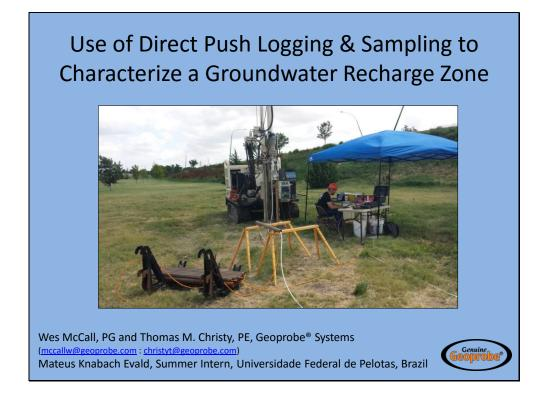
Basic field set up for conducting HPT-GWS logging/sampling near the N. Ohio bridge. "Matt" worked with us as a summer intern. The original purpose of our project was to test the new 20 port HPT-GWS probe and sampling system. During our field testing we learned some unexpected details about the subsurface aquifer in this area.
