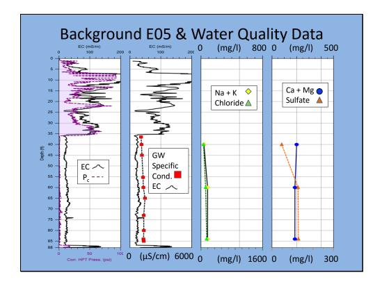
Groundwater specific conductance measured at several depths across the aquifer gives a pretty flat profile, much like the EC log. Also, the cations and anions all give pretty flat concentration profiles across the aquifer at this location, similar to the EC log. Boring .....
