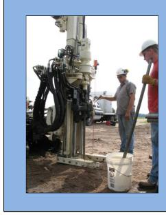
The hydraulic hammer, hydraulic slides and vehicle weight are used to advance the tools into unconsolidated materials.
