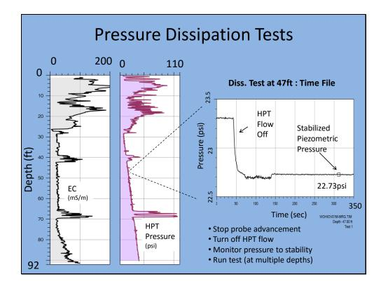
Dissipation tests are usually performed in low EC, Low HPT pressure zones (coarse grained) so that pressure dissipation occurs quickly. If you attempted a pressure dissipation test at 17ft at this location (higher EC and pressure) it may take several hours (even days) for the pressure to dissipate. The dissipation test shown here was run at 47ft in the low EC and low HPT pressure materials. The stabilized pressure here tells us what the piezometric (hydrostatic) pressure is at this depth.
