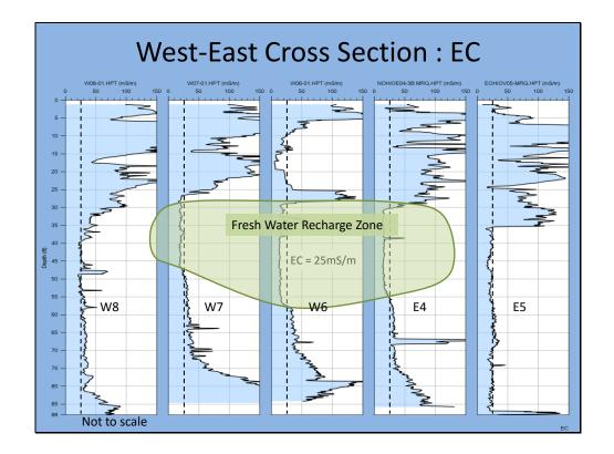
Shading is applied here to help visualize the fresh water recharge zone in the upper part of the sand/gravel facies (the aquifer). Again, defined as the zone in the saturated sand and gravel where bulk formation EC is below 25mS/m.
