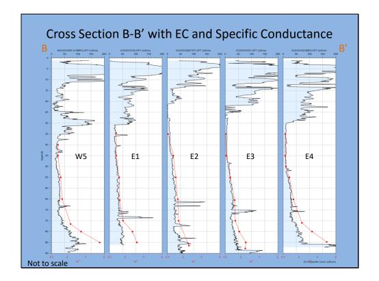
Here is the cross section of logs with EC shaded blue and groundwater specific conductance in red line with red square. First ... As we have seen the upper facies of the formation is comprised of high EC fines (clay) with varying amounts of silt and sand. The thickness of this fine grained facies varies across the site.
