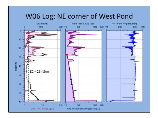
At this location the corrected pressure (left panel) below 28ft indicates the formation is mostly high permeability sand and gravel with a clay layer between 32-34ft and a clay lens at about 67ft. Pressure and EC increases at 78ft defines the top of the shale bedrock at this location. Bulk formation EC from 29-~56ft is below the background average, indicating freshwater recharge. Below ~70ft the EC trends up indicating brine impact.
