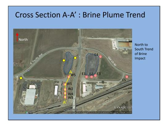
Let's look at a cross section (A-A') of the EC logs together with the groundwater specific conductance data to asses the concentration trend ~north-to-south across part of the brine plume.
