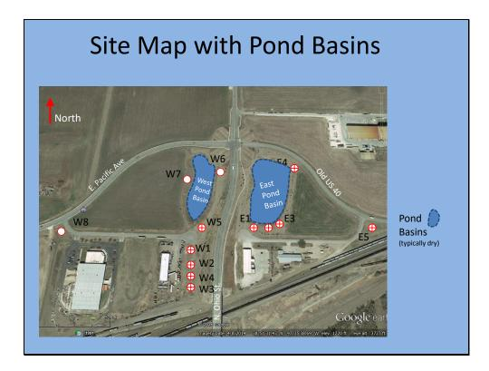
Note the two pond basins here. These were constructed to catch storm water runoff and provide a nice esthetic view along the road into town. Unfortunately the ponds only have a little water in them immediately after a rain storm, otherwise they are dry.
