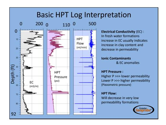
At this location the upper 25+ft is dominated by high EC and elevated HPT pressure, so primarily a lower permeability, finer grained facies.
