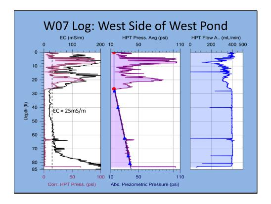
Results here are similar to the W06 location just discussed, but the low EC area does not go as deep nor as low as in the W06 log. Conversely the EC readings at depth (below 70ft) due to the brine are higher. HPT pressure defines top of shale at just below 82ft here.
