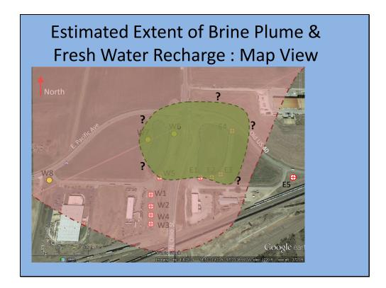
Here the green shading (over the pink) is used to estimate the aerial extent of the fresh water recharge in the upper part of the aquifer. The south edge appears to be close to the W5 and E1 logs based on the bulk formation EC at those locations. Alternately, the north side of the recharge plume may extend further north, more logging data would be required to accurately define the full extent of the fresh water plume.
