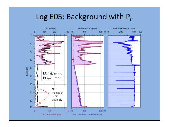
Let's focus on the EC and corrected pressure log here (left panel). Above 35ft we have high EC and pressure, so fine grained facies with varying amounts of silt and sand. Below 35ft both EC and  $P_c$  are flat and featureless so no indication of brine impact in the lower part of the formation as seen in the W01 log. Note the EC and Pressure peaks at the top of the shale at ~87ft. Let's look at some water quality data for this location.
