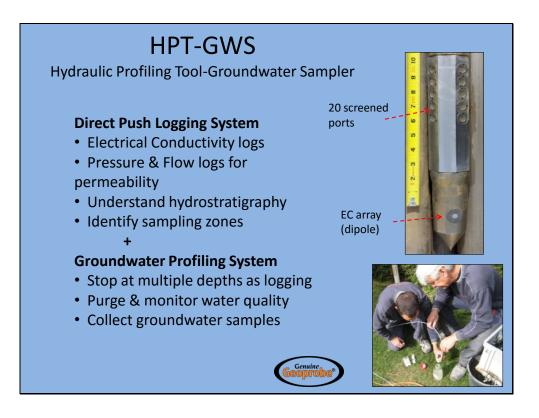
We used the HPT-GWS system to conduct the logging and sampling for this project. This is a DP logging system and a DP groundwater profiling system in one tool. DP tools are for penetration of unconsolidated soils and sediments. These tools will not penetrate consolidated rock.
