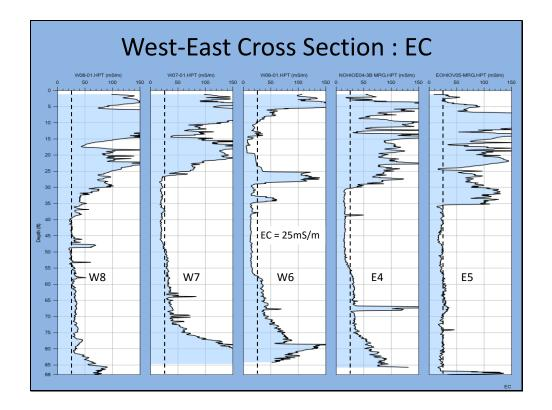
Now on the cross section (not to scale), plotting the average background EC for the saturated sand/gravel facies over the logs again allows you to see where the bulk formation EC is low (fresh water recharge) and the bulk formation EC is high (brine impact) for all of these logs.
