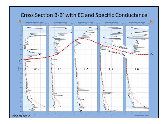
Here a red dashed line indicates the base of the clay rich facies based on EC dropping to 50 mS/m. It is apparent that the clay rich facies is thinnest at the E2 log location. Below the upper facies and above 75ft the formation is mostly lower EC sand & gravel with a few clay layers, often in the 65-75ft zone. Then down around 75ft we see increases in EC due to our EC anomaly (elevated specific conductance) that we already observed in other logs at the site.
