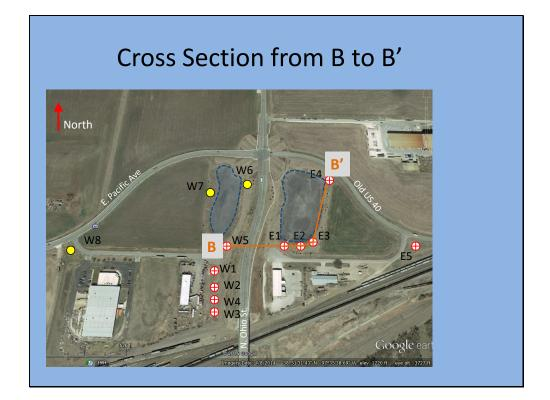
Let's look at a cross section from B (at W5) to B' (at E4) to evaluate the 3 zones of water quality. Note lateral spacing between the logs is not equal here but the logs in the following cross sections are presented with equal spacing, so not to scale laterally, but very useful for identifying water quality zones.
