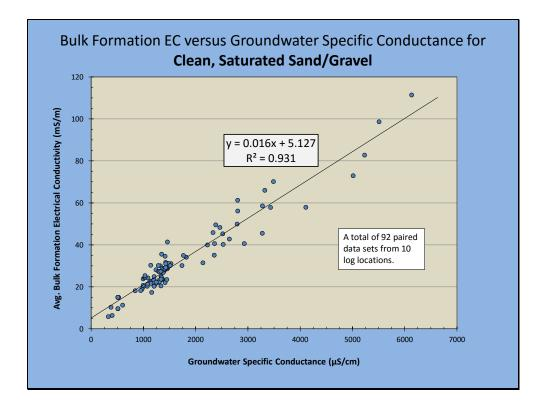
With a little spread sheet work we see that there is a strong correlation between groundwater specific conductance and bulk formation EC for the clean, saturated sands/gravels. So this gives us a site specific model to help identify EC anomalies at this site. This model may have some potential for use as a general model for sites with similar conditions but more data would be needed to confirm that. At sites with very concentrated brines a different model would probably be required.
