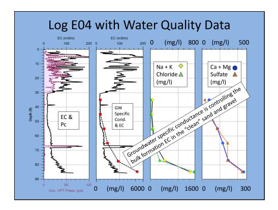
And the groundwater specific conductance is controlling the bulk formation EC in the saturated, clean sand and gravel facies. (Excluding clay-rich lenses and layers.)
