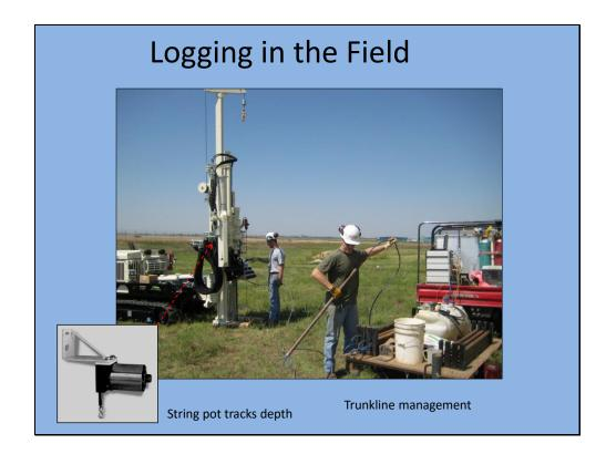
A probe machine advances the tool string into the subsurface while a stringpot tracks depth of the probe. Rod and trunkline management provide your daily workout routine. The trunkline is pre-strung through all of the rods before logging is started to make the process efficient. The trunkline attaches to the up-hole pump and electronics, including a lap top computer to display the log data.
