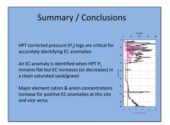
The results presented here reveal that the combined HPT pressure and EC logs can provide a very useful tool for use in selecting locations for construction of aquifer recharge basins in unconsolidated formations.
