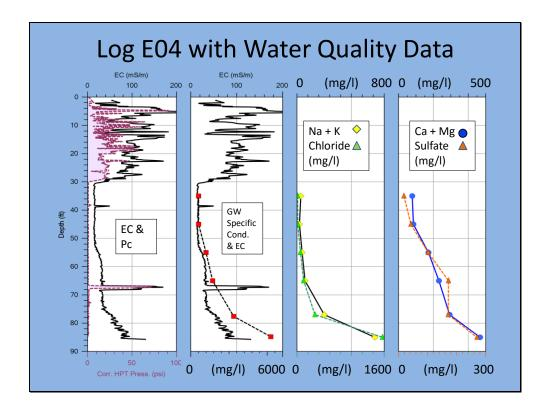
Much as we expected the Groundwater specific conductance, cation and anion concentrations are low in the upper part of the aquifer and increase some near the middle and are noticeably higher below 75ft where we observe the positive EC anomaly. So we see that the dissolved ion concentrations are controlling the groundwater specific conductance.
