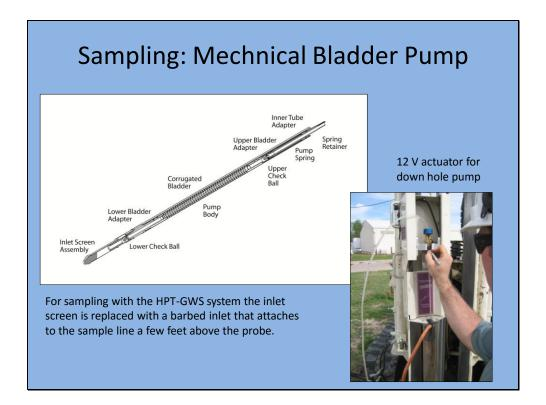
A 12V electric actuator mounts on top of the 2.25" tool string and the sample line is attached to the slider block. The up and down motion of the actuator opens & closes the bladder in the pump, pumping water to the surface. Depending on depth and formation permeability flow rates range between 50ml/min and 300ml/min. Low permeability formations (high EC and high HPT pressure) will not yield water for sampling. For more information about the pump go to www.geoprobe.com
