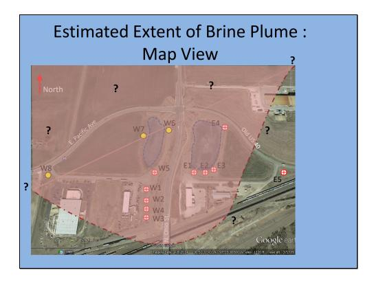
Based on the limited data from the EC logs versus HPT Pc logs this gives an estimate of the extent of the brine plume around the area studied at this time. The closest municipal supply wells are about 1.5 miles south of this area. More logs would be required to further constrain the extent of the brine plume.
