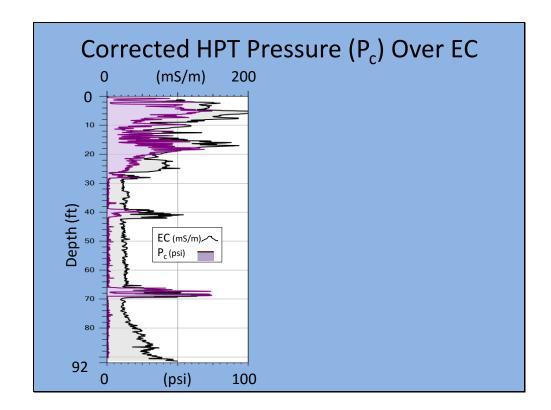
We can plot corrected pressure over the EC log to see how they compare. In the upper 25+ft we have high EC and high pressure = low permeability. Below 30ft Pc and EC are generally low, with both increasing when clay layers are encountered. But what is going on below 75ft?
