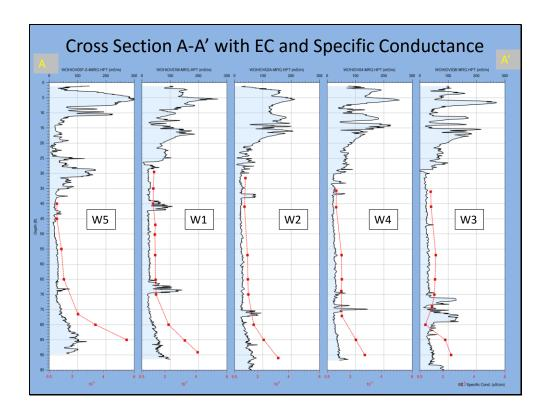
The logs all show EC increasing below 70-75 feet but as we go south (to the right toward A') the increase in EC below 75 feet diminishes. A similar trend is displayed by the specific conductance of the groundwater samples. This indicates that the brine source is probably north of the study area and the impact of the brine is generally decreasing to the south in this area. Of course additional logs and water quality data would help to substantiate this data and interpretation.
