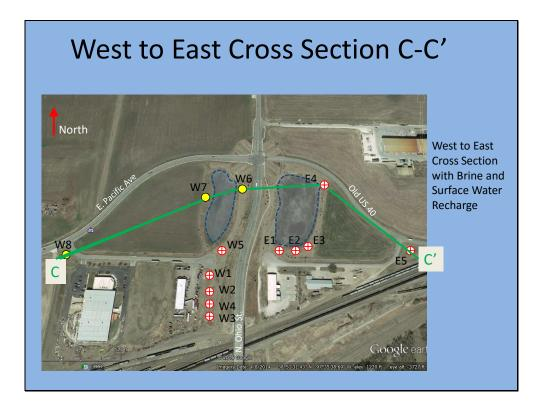
Let's look at a west-to-east cross section (C to C') of the EC logs to assess the extent of fresh water recharge and the brine plume in the study area. First, let's review logs W6 and W7 to evaluate the EC relative to corrected HPT pressure.
