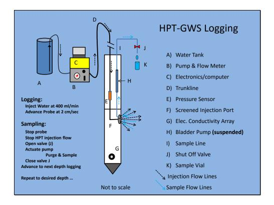
The pump in the HPT flow module (B) draws water from the supply tank (A) and pumps water down the trunkline (D) at a constant flow rate. An inline flow meter (B) measures the flow rate. The downhole pressure sensor (E) monitors the pressure required to inject water into the formation matrix. The HPT-GWS probe includes an electrical conductivity (EC) array (G). The EC, pressure and flow rate are logged every 0.05 ft (~15 mm) and displayed onscreen as the probe is advanced.
