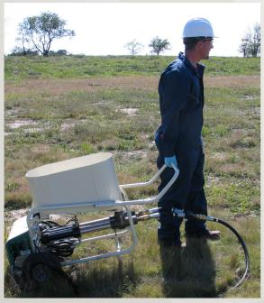
Weighing less than 150 lb., the GP350 can be loaded by two people and can be easily maneuvered around a project site by one field person.
