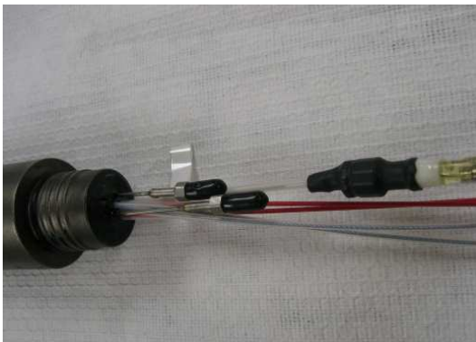
Fig. 12: Heat shrink around thermocouple connection
