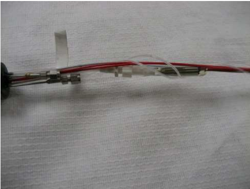
Fig. 5: Wrapping excess gas line around wires
