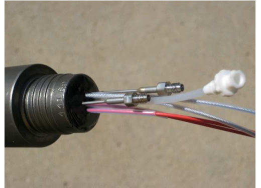
Fig. 9: Gas lines and thermocouple duct
