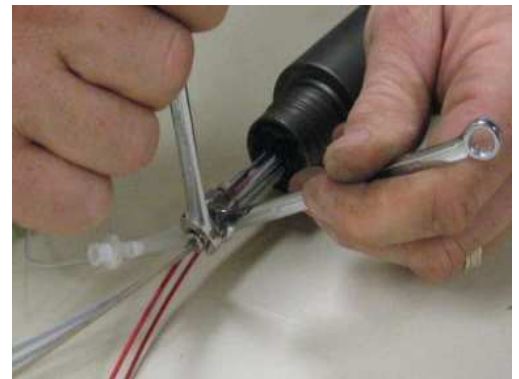
Fig. 7: Connecting the trunkline gas lines to the probe
