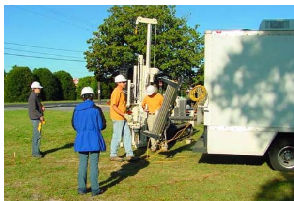
(above) Green Services of Bel Air, MD, provided the 6620DT and partnered with COLUMBIA Technologies to conduct the MIP investigation to pinpoint TCE contamination. (left) By using SmartData Solutions®, a rapid 3D visualization and information delivery system developed by COLUMBIA Technologies, coupled with the MIP data, the field team was able to optimize specific results from the site in real time in the mobile, onsite field office.
