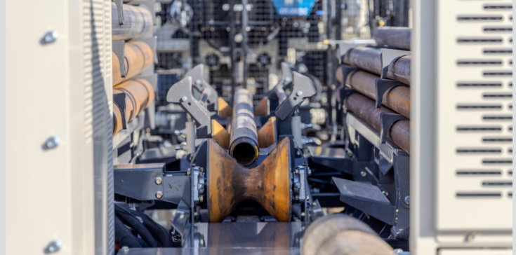
Carriage comes with reversible live rollers, simplifying the loading and unloading process.
