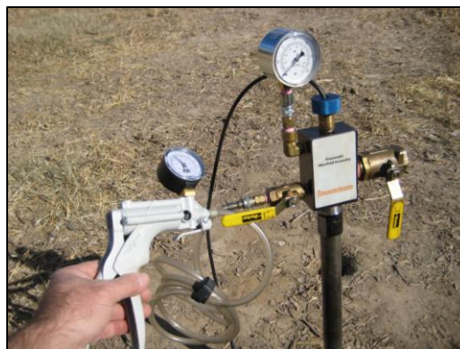
Figure 13: Setup for leak test and rising head tests with the pressure gauge and hand pump. The gauges are graduated in inches and centimeters of water pressure (outer and inner marks respectively). Close the inlet valve after pressurizing.
