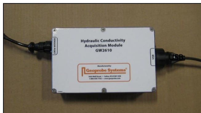
Figure 6: The USB cable and transducer cable are connected to the GW2610 Acquisition Module (214040).
