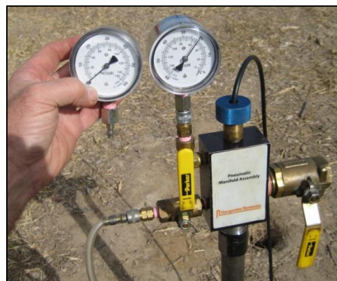
Figure 13: Use the vacuum gauge to perform falling head tests or install the pressure gauge to conduct rising head tests and for leak testing.
