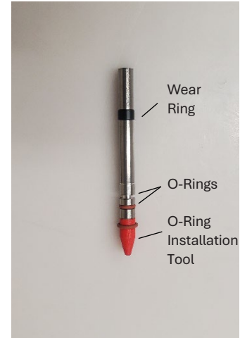
Figure 5.4: Syringe Pump Piston with O-Ring Installation Tool
