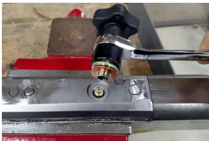
Figure A.3.1: Unthread the membrane from the probe block and make sure the copper washer is also removed and replaced with the membrane.
