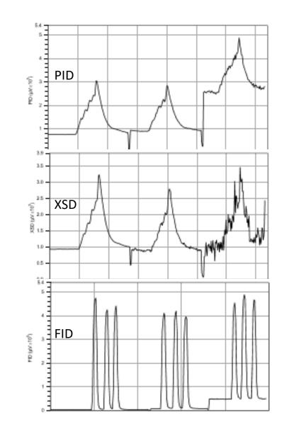
Gain Adjustment Test on the SRI PID and FID and the OI XSD.
