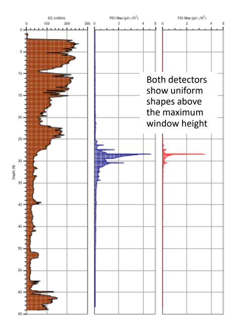
This is an example of a test of the detector gain adjustments.
