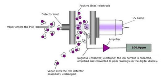
Photoionization Detector (PID)
