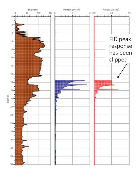
To avoid peak "clipping" the detector gain can be adjusted down by the operator. This divides the detector signal by some factor -10 for example.
