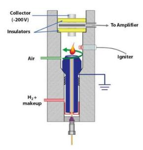
Analytes in the MIP carrier gas stream are combusted in a hydrogen flame, creating positive ions and electrons. The positive ions are attracted to the negatively-biased collector while the (negatively charged) electrons are repelled toward the jet.
