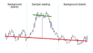
Detection Limit is defined as signal that is 3x higher than base line noise
