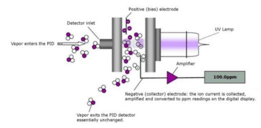
Photoionization Detector (PID)
