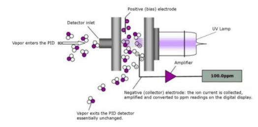
Photoionization Detector (PID)
