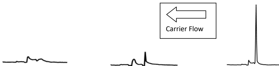
Figure 10: Example peaks where the Vent time is set too short – the peak is being cut off by the valve switching.
