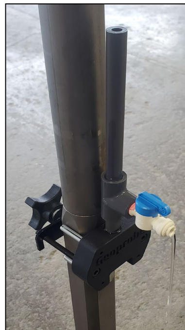
Figure 5.10: HPT Reference Block Setup
