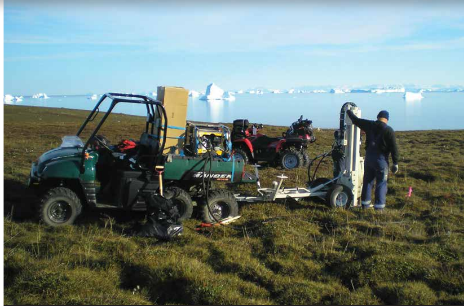
A 540MT is used for geotechnical surveys at a potential mining site in Greenland.
