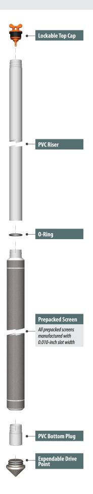
Designed for setting small diameter groundwater monitoring wells, prepacked screens consist of a standard, slotted PVC well screen pipe surrounded by a stainless steel mesh. Sand is prepacked around the slotted PVC before the well screen is installed, guaranteeing sand will be located directly around the well screen for quicker more efficient groundwater monitoring well installation.
