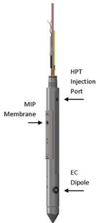
Figure 1. The MiHpt probe body is 520 mm (20.5 inches) long and about 45 mm (1.75 inches) in diameter. The heater block at the MIP membrane is heated to 100 °C to enhance VOC diffusion from the formation across the membrane.
