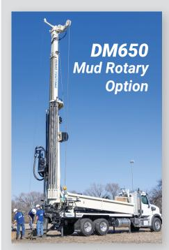
Simplified mud or air drilling suited for geotermal, water well, or irrigition projects, the DM650 is easily mobilized from job site to job site.
