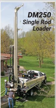
The helper side controls to operate the jib and winch functions make the DM250 easy to operte with a two-man crew while minimizing movement of the top head for faster production.
