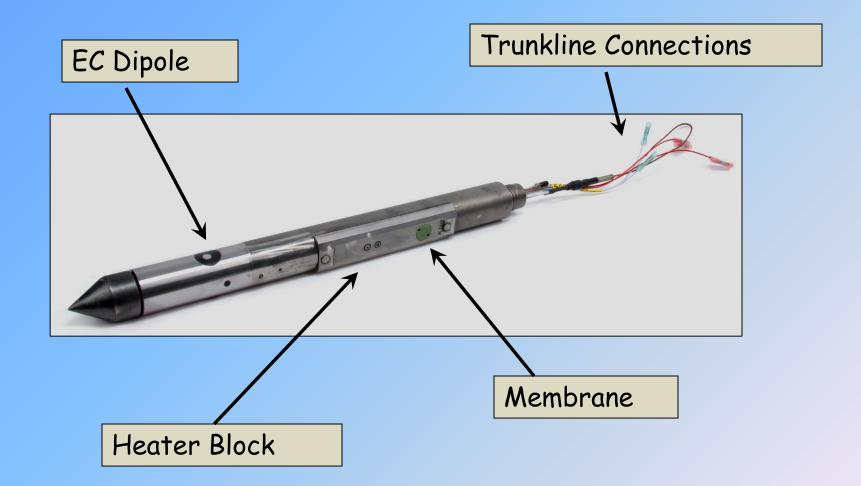
The heater block heats up to 120C to help "extract" volatiles from the formation. The thermocouple is used to monitor & control the temperature. Supply and return gas lines in the trunkline connect to the fittings at the probe.
