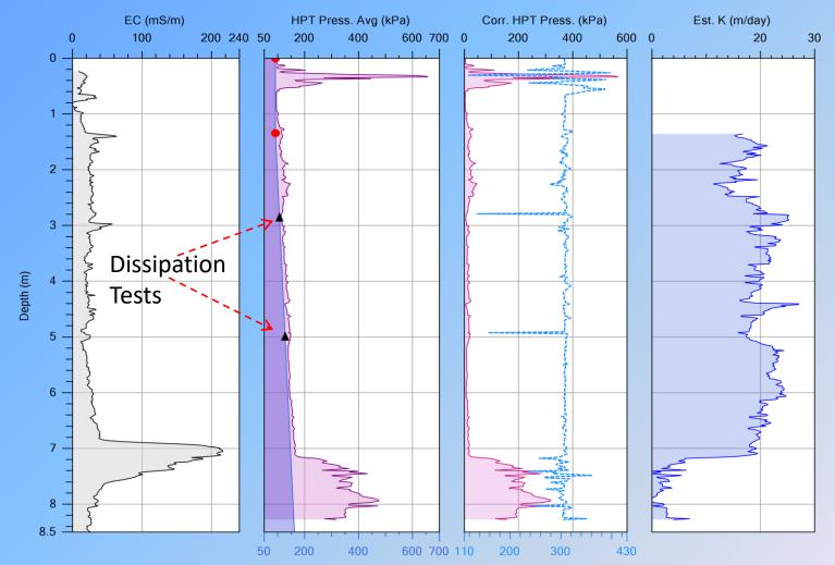
As you advance below the water table hydrostatic pressure effects the HPT pressure measured. Dissipation tests are used at selected depths to determine the piezometric pressure. Once we have the potentiometric profile that pressure can be subtracted from the total HPT pressure to determine the corrected HPT pressure.
