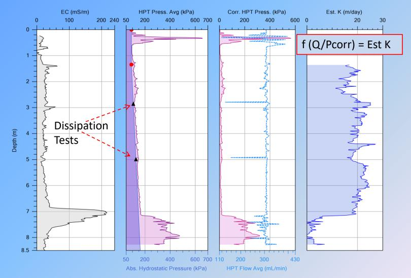
The corrected HPT pressure is the pressure required to inject water into the formation. The corrected pressure and flow are then used in an empirical model to calculate the estimated hydraulic conductivity of the formation at the inch-scale.
