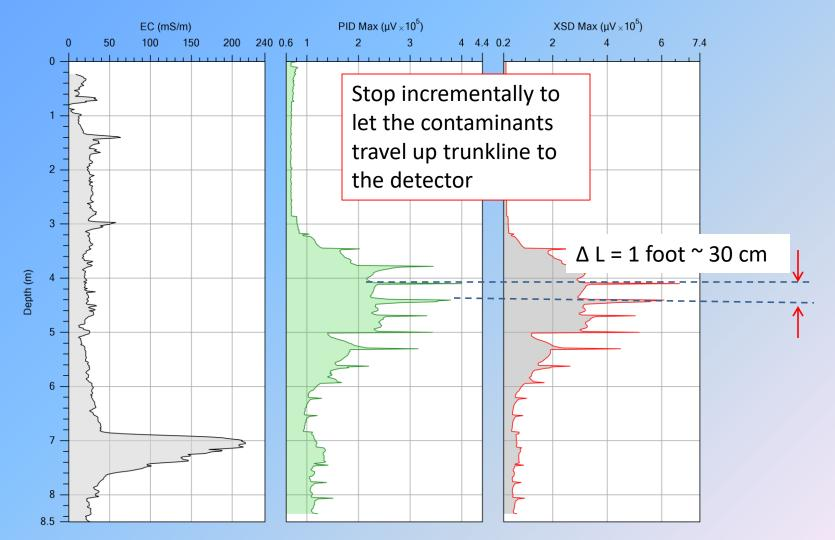
The peaks or "spikes" in the detector logs are caused by the incremental probing. Stopping at each depth interval for about 45 seconds to allow time for the probe to reach temperature and diffuse contaminants across the membrane.
