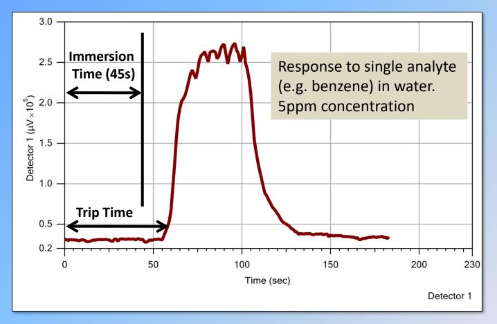
Trip time is the time required for analyte to travel across the membrane and through the trunkline to its first observation at the detector. The trip time is entered into the software to allow for accurate tracking of contaminants in the log.
