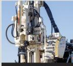
Geotech Head Assembly & Automatic Drop Hammer
