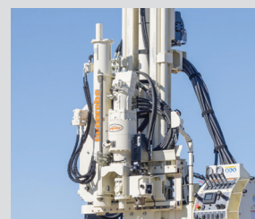
Geotech Head Assembly & Automatic Drop Hammer
