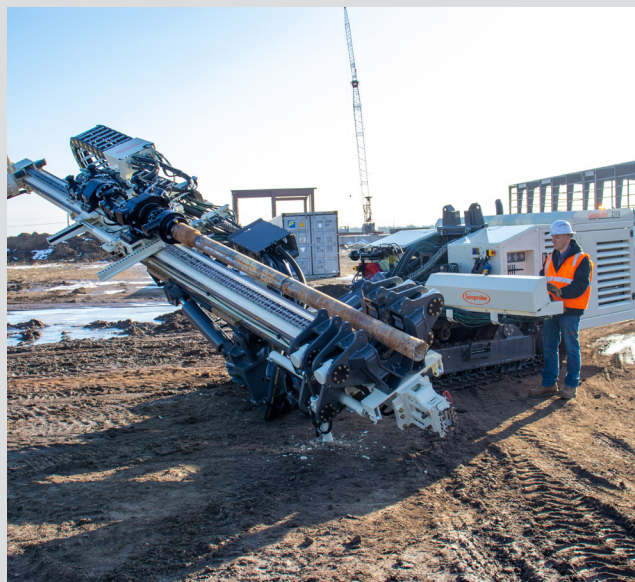
Front-the-wall kinematics provide versatile mast positioning, making the 21FH an efficient tieback rig.
