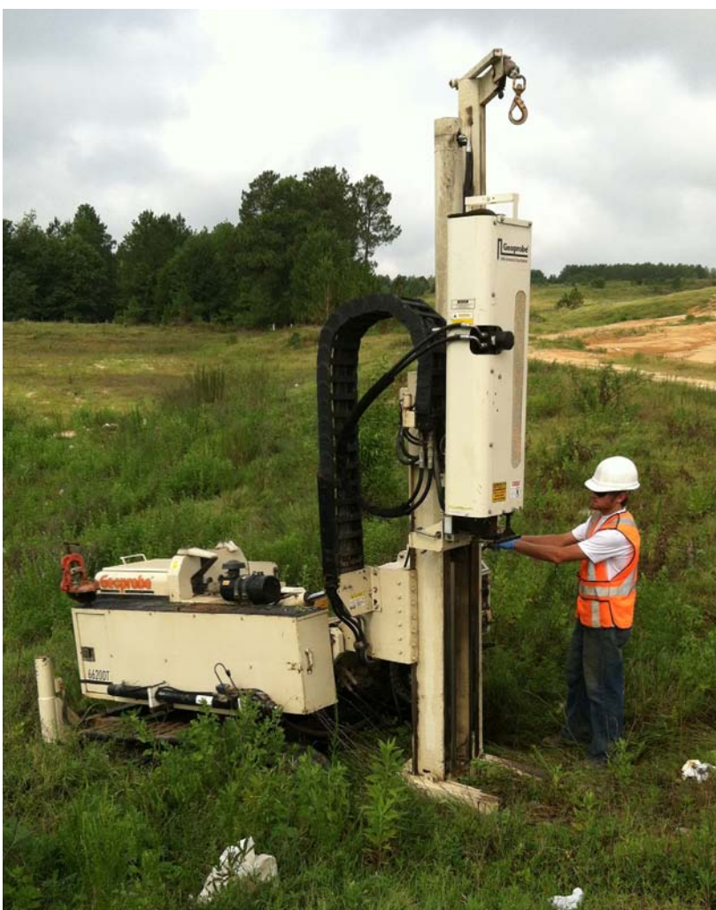
Chas McLaughlin, Environmental Technician for Elite Techniques Inc., pushes a Macro-Core® soil sampler to 65 ft. on a slope hill at the Kershaw County landfill.
