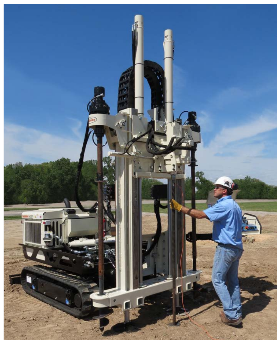
Tom Christy of the Geoprobe®-DI Team uses a 6622CPT platform for FFD logging (Fuel Fluorescence Detector) at the Geoprobe® Open House event. The 6622CPT rig is a special purpose machine that shares a common chassis with the popular Geoprobe® Model 7822DT. The front end of the 6622 is a 20-ton, self-anchoring push platform complete with a hydraulic chuck (located between the push cylinders). For this photo, the machine is unanchored and an FFD logging tool is being driven to depth using the GH64 hammer, that is standard to the 6622, and is useful for driving samplers or percussion driven logging systems.
