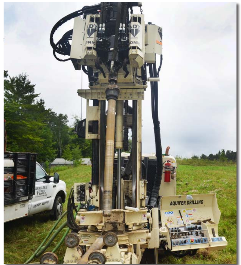
The ADT field team used 6 in. casing with the Geoprobe® 8140LC for soil core collection and for installing multi-level wells.
