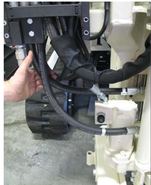
To prevent the hammer lines from sliding down through the hose carrier, the new Hammer Lines Kit splits the hammer lines into two pieces.
