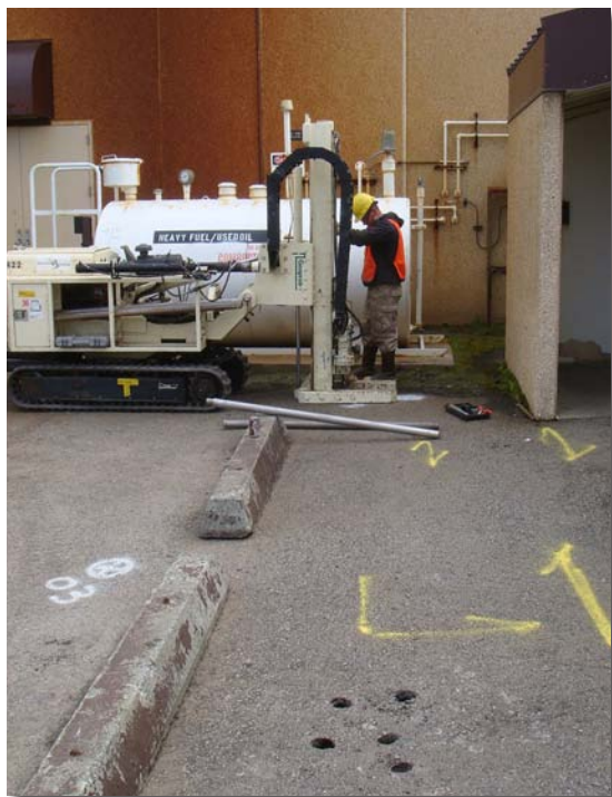
Three, four, or even five adjacent borings (five are shown in the foreground) were in process simultaneously in order to provide enough soil redundancy at specific depths for the lab to analyze.
