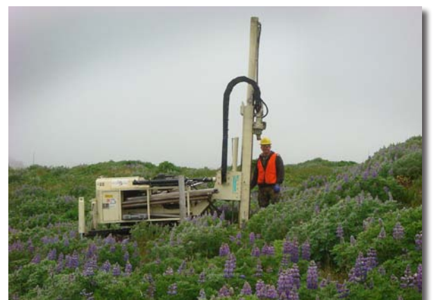
The relatively small size of the Geoprobe® 66DT makes it well suited to ship to remote areas of Alaska, such as Kotlik, Barrow, Quinhagak and Atmautluak. Here, soil samples are collected at this site on Shemya Island.
