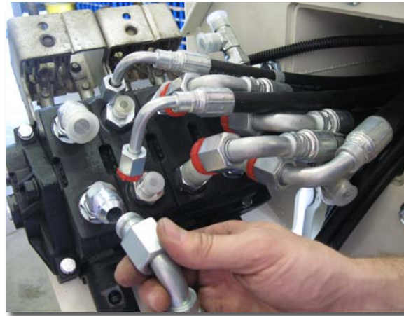
(above) Roman Burrows, Geoprobe® Service Specialist, feeds replacement hoses in the new Hose Carrier Kit for a 6620DT through an opening to the control panel. (left) All hoses in the Hose Carrier Kit are cut the correct length easily connect to Valve Body on the back of the control panel.
