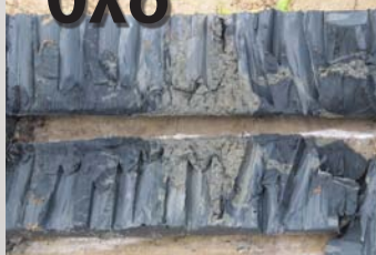
6x8 silt samples collected using a Geoprobe® 8140LS in Georgia. The material was likely dredged out of a nearby waterway.
