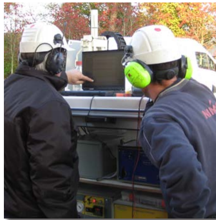
A field team in Denmark review MIP detector results and HPT pressure log onscreen as the MiHpt probe is advanced. Having the HPT pressure log along with the detector results is useful in understanding how the lithology controls contaminant migration.
