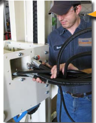
(above) Roman Burrows, Geoprobe® Service Specialist, feeds replacement hoses in the new Hose Carrier Kit for a 6620DT through an opening to the control panel. (left) All hoses in the Hose Carrier Kit are cut the correct length easily connect to Valve Body on the back of the control panel.
