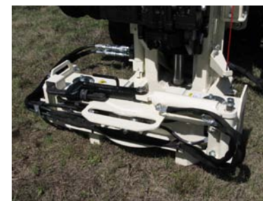
The 7822 Series 6-in. single clamp breakout.
