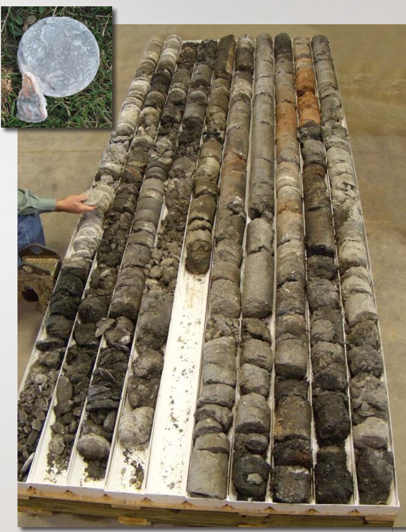
Mike Carlin (left), Jed Davis, and Dave Golden (with camera), Geoprobe® Tooling Engineers, test new Geoprobe® DT60 sonic tooling by collecting 200 ft. of 6.0 in. cores using a Geoprobe® 8140LS and Geoprobe® sonic tooling. Kansas wind chills during the test period were 0 degrees.
