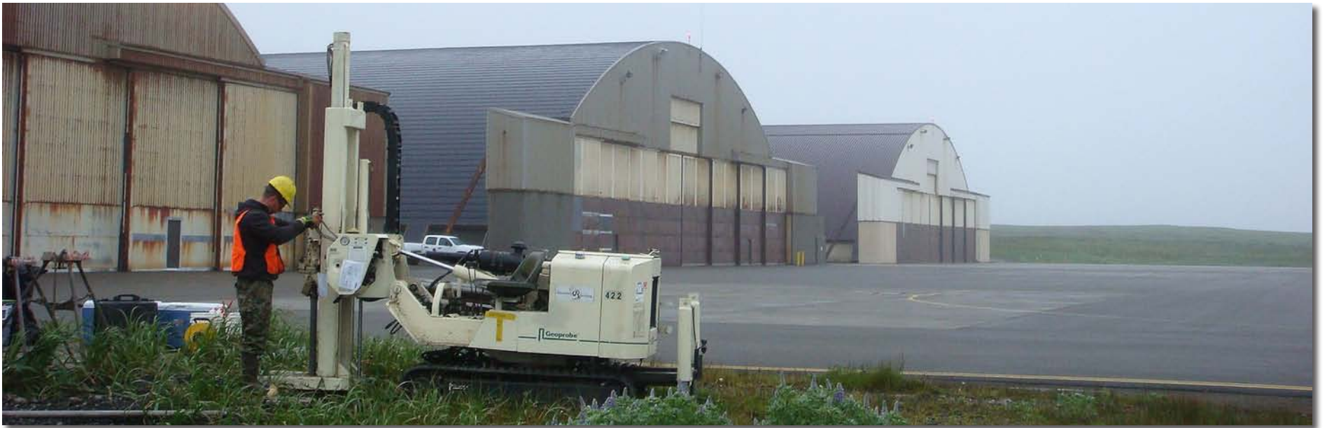
DJ Wardwell, Assistant Operations Manager for Discovery Drilling in Anchorage, AK, uses a Geoprobe® 66DT to pull soil samples near some abandoned fuel storage tanks at Eareckson Air Station on Shemya Island.
