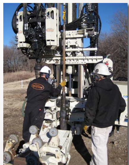
Mike Carlin (left), Jed Davis, and Dave Golden (with camera), Geoprobe® Tooling Engineers, test new Geoprobe® DT60 sonic tooling by collecting 200 ft. of 6.0 in. cores using a Geoprobe® 8140LS and Geoprobe® sonic tooling. Kansas wind chills during the test period were 0 degrees.
