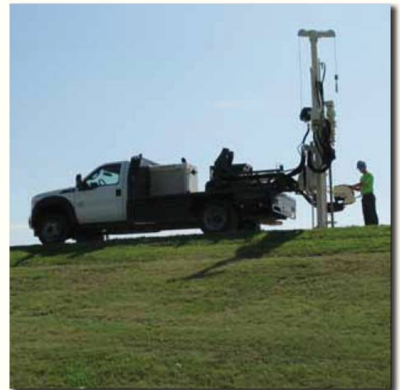
Soil sampling at a flood retention dike with the 7800.
