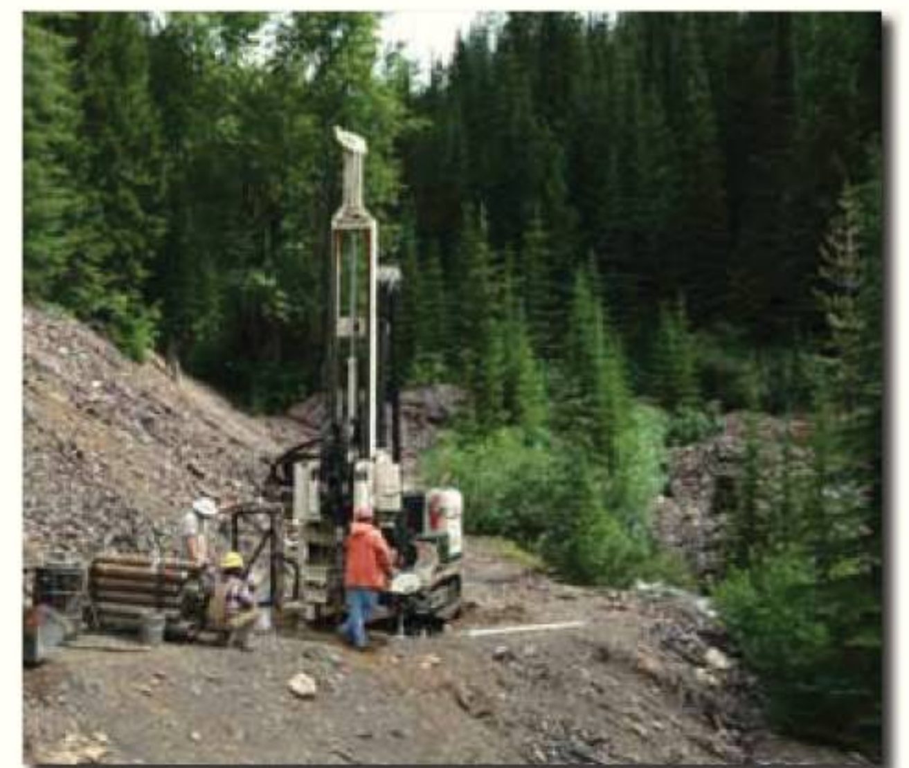
(above and below) MDE field team with 8140 Rotary Sonic for remote sonic drilling within mine rock dump in northern Idaho.
