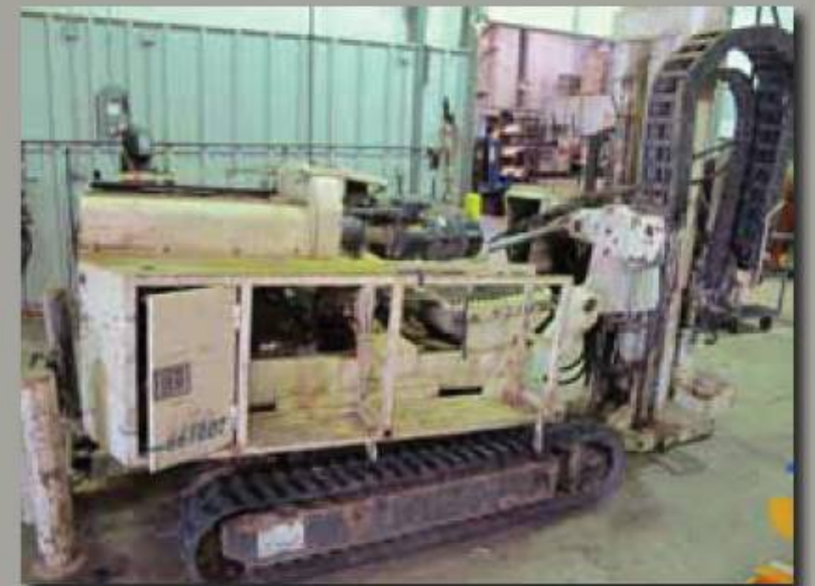
GH64 Hammer (shown here with GA4000 Augerhead) comes standard on 78 Series rigs.
