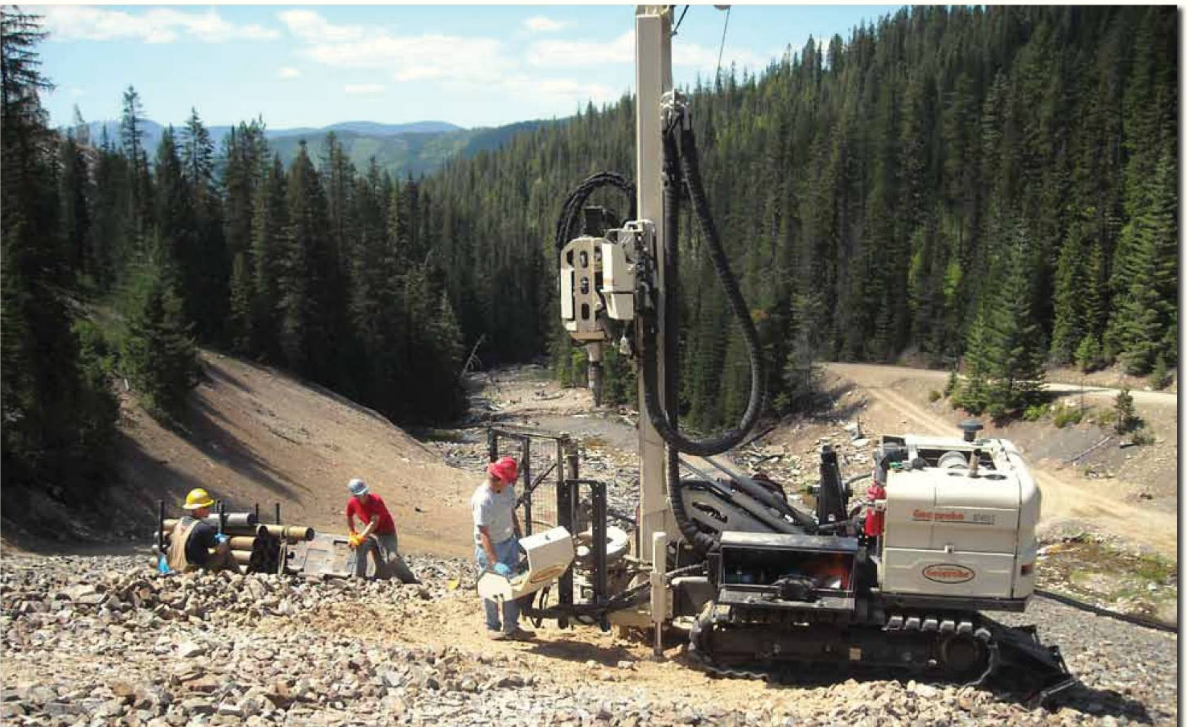
(above and below) MDE field team with 8140 Rotary Sonic for remote sonic drilling within mine rock dump in northern Idaho.
