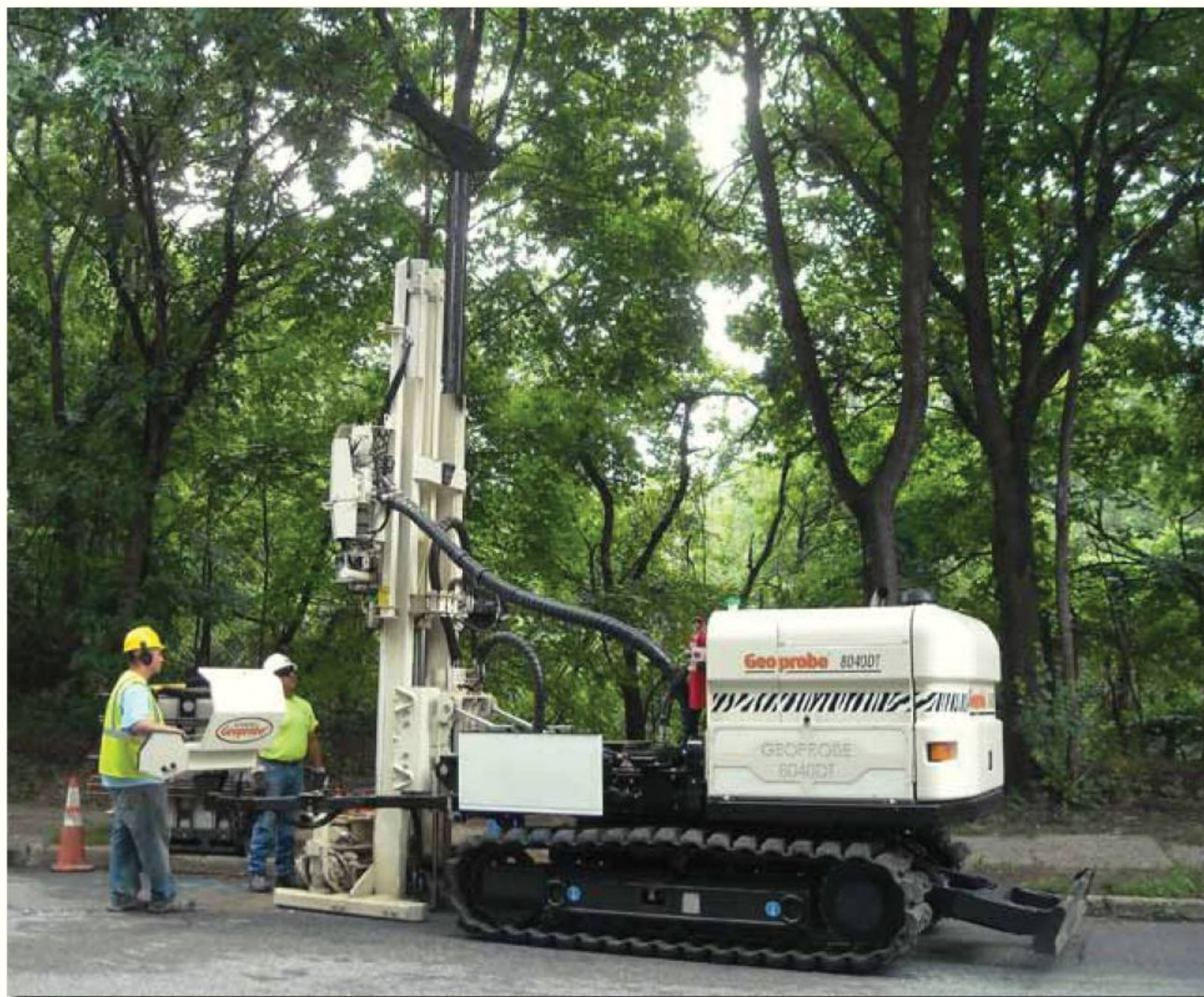
(l to r) Evan Moraitis and Jose Garcia were part of the ZEBRA Environmental field team on the Solvent Finishers site. ZEBRA used the 8040DT at the site because of its direct push capabilities and also quick set up time, usually about 20 minutes.
