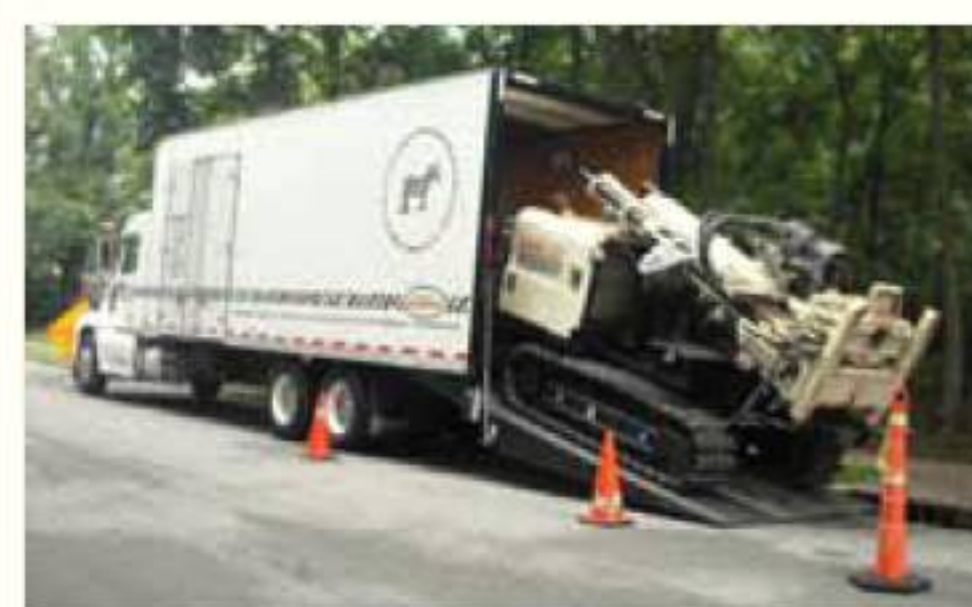
(above) ZEBRA Environmental's truck was designed specifically to transport their 8040DT and onsite supplies and equipment. (left) The Geoprobe® 8040DT features a Drop Rack System allowing the rig to carry tooling to the site on the rear blade. (right) More ZEBRA information on page 19 ... 100 Club.
