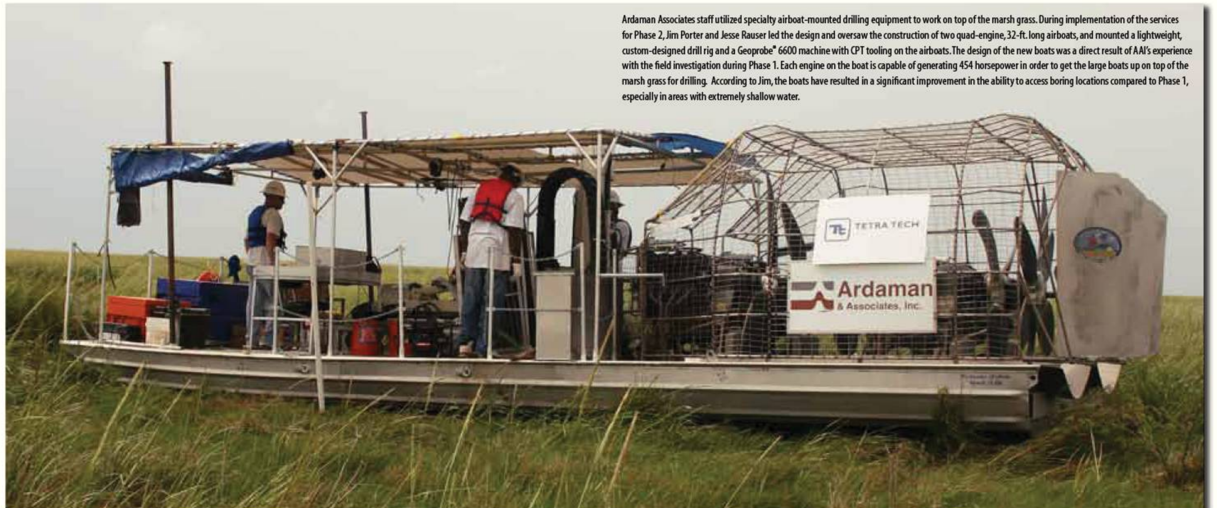
Ardaman Associates mounted a Geoprobe® 540UD in a smaller airboat for a 2003 project. The most recent work completed in Lafourche Parish in Louisiana required an airboat with more than twice the power of the above configuration.
