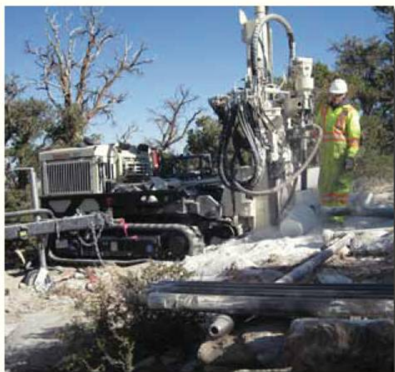
Gregg Drilling in Signal Hill, CA, use a 7822DT while running a 4-in. downhole hammer looking for limestone near Big Bear Lake, CA.
