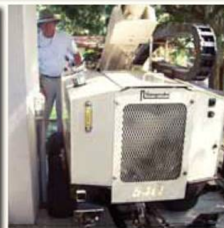
(top) Glen Doran, Professor, and Bruce Albert, a pollen specialist, work with the Geoprobe® 54LT, owned by the Florida State University Department of Anthropology. The machine operates with wheels instead of traditional tracks, and is pulled by a Honda Foreman ATV. The rig has been used on over 30 archaeological sites in Florida, Tennessee, Louisiana, and Texas. (left) Glen Doran, Professor, watches as Grayall Farr, Geoprobe® technician, prepares to collect a soil core sample. (center) Sometimes FSU collects only one or two cores at a site; in other cases, 5 to 50 cores are taken, some of which are immediately sliced open and examined. (right) With a width of 35 in., the 54LT can squeeze through openings to access confined areas. John Foss, geoarchaeological consultant, helps guide the machine through a residential gate at the Bay West site on the Florida Gulf coast.
