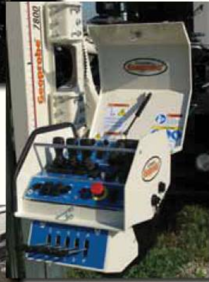
Control Panel with Integrated Electronic Diagnostic System, standard for 7800
