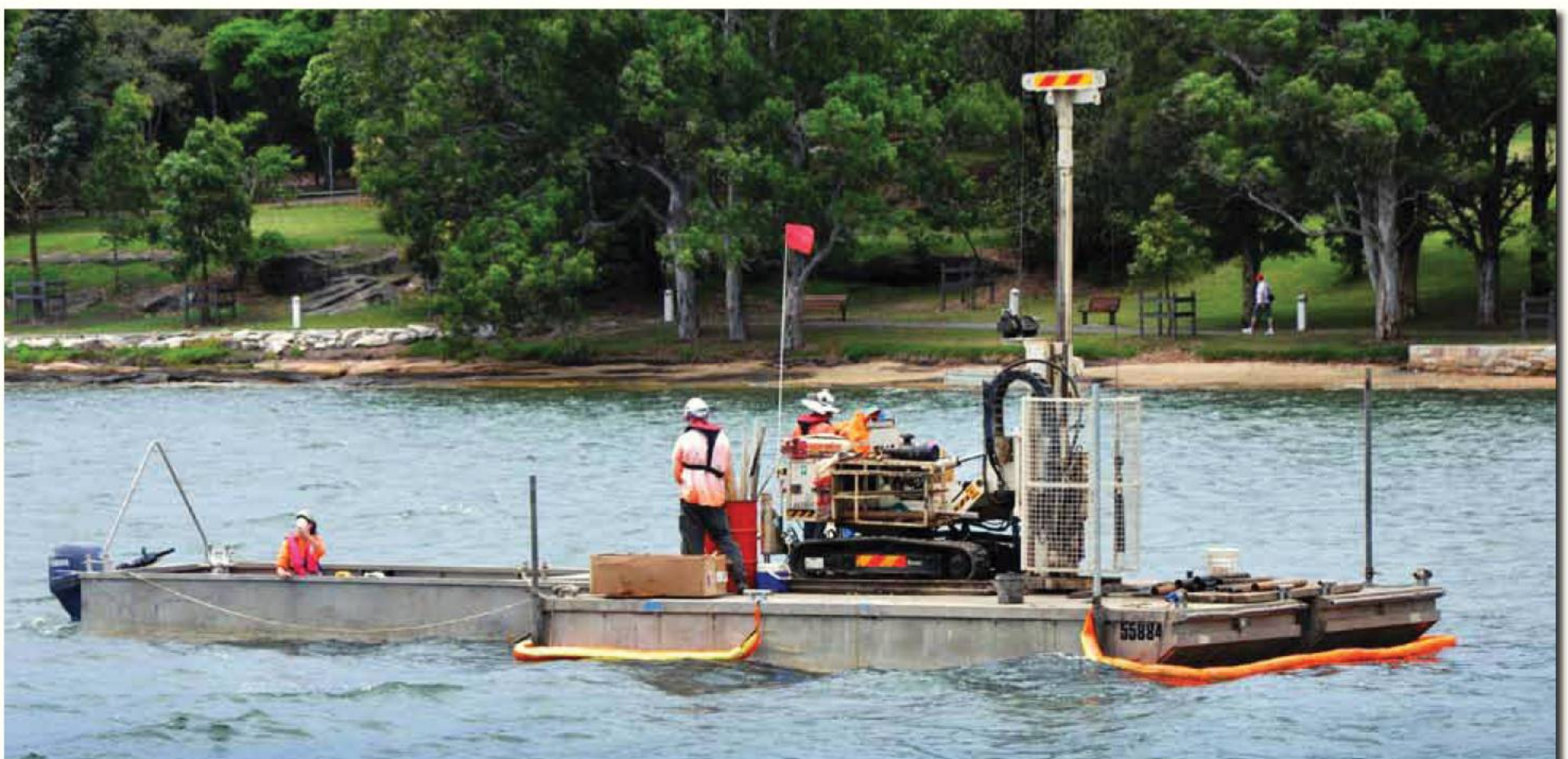
The experience of the Terratest crew and the ease-of-use of the DT325 tooling with the 6620DT kept the work moving along quickly. The sediment was completed ahead of schedule resulting in earlier reporting of the findings and significant cost savings to the client.
