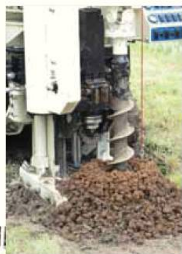
Rotation speed of the GH64 hammer was designed to turn larger diameter augers.
