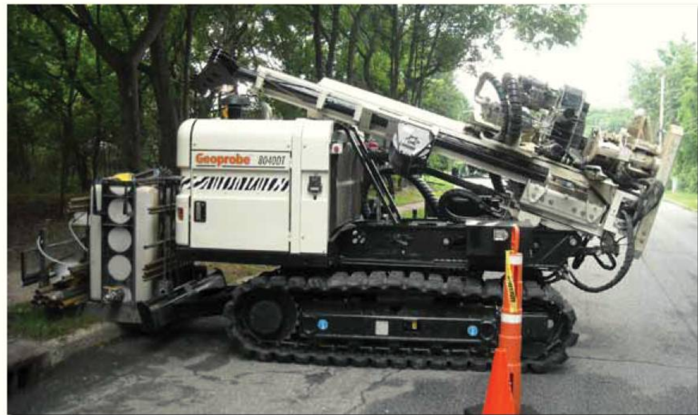
(above) ZEBRA Environmental's truck was designed specifically to transport their 8040DT and onsite supplies and equipment. (left) The Geoprobe® 8040DT features a Drop Rack System allowing the rig to carry tooling to the site on the rear blade. (right) More ZEBRA information on page 19 ... 100 Club.
