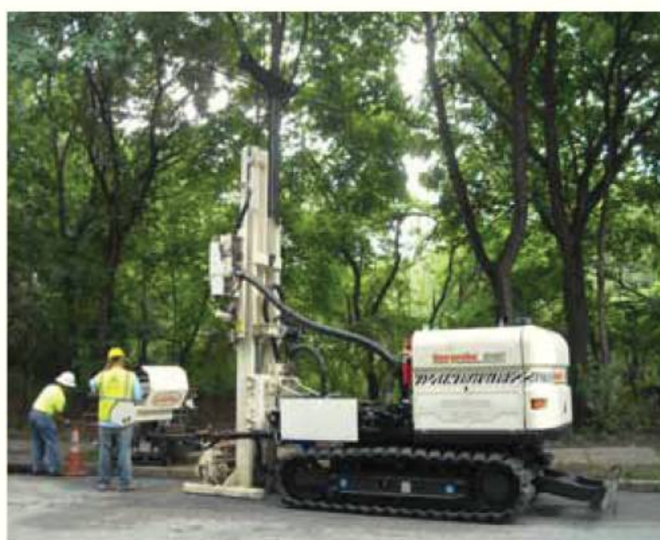
Chris Lacko, Field Operations Manager for ARS Technologies in New Brunswick, NJ, uses their 8040DT at an abandoned manufacturing facility, continuous coring with DT325 tooling to over 100 feet.
