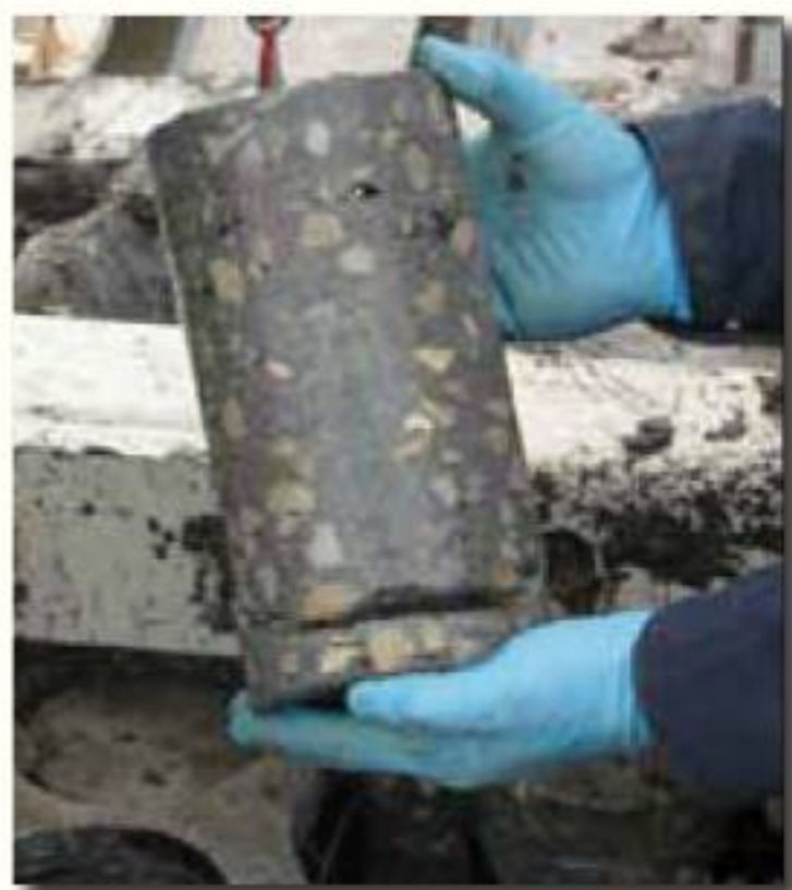
Concrete coring applications can now be completed using 78 Series rigs. (left) A 5-in. concrete core opens up the subsurface for sampling or monitoring well installation.
