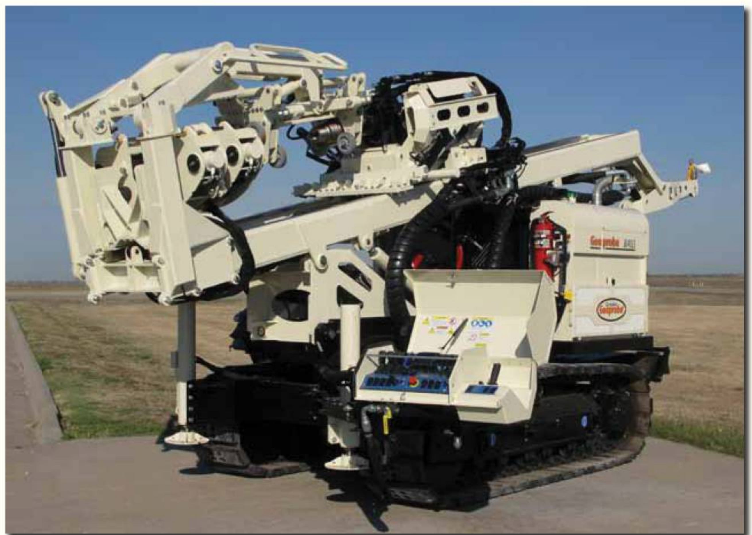
The 8140LS equipped with an option Rod Handling System.
