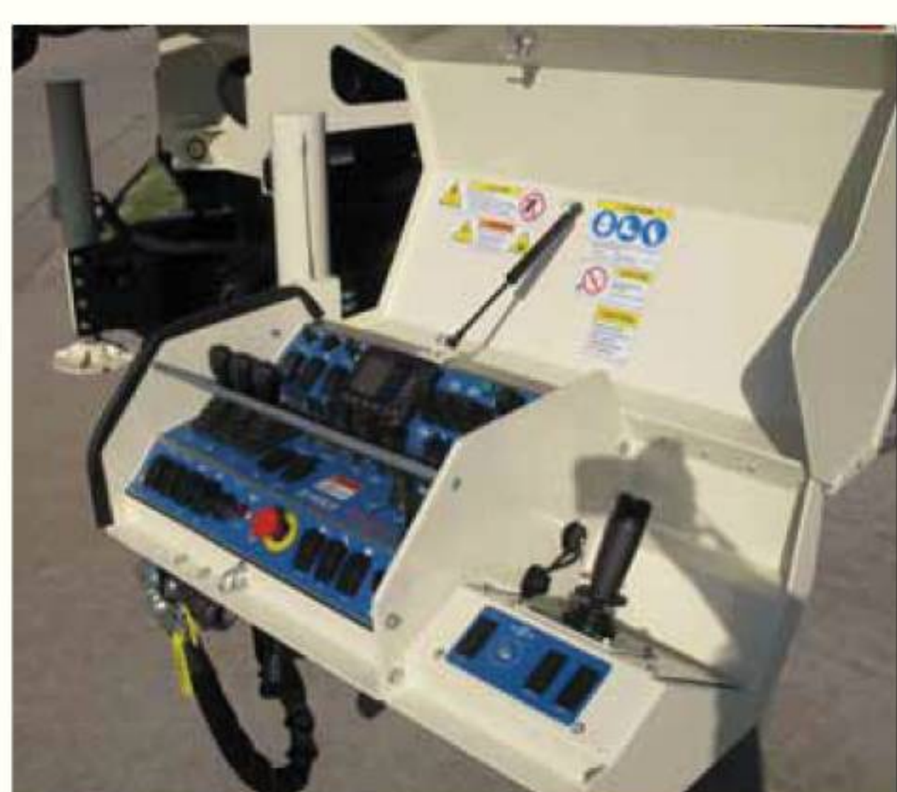
The operator-adjustable control panel on the 8140 rotary sonic series rigs features a well-organized, easy-to-learn control layout.
