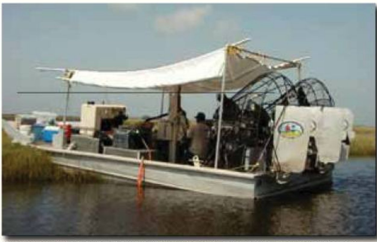
Ardaman Associates mounted a Geoprobe® 540UD in a smaller airboat for a 2003 project. The most recent work completed in Lafourche Parish in Louisiana required an airboat with more than twice the power of the above configuration.
