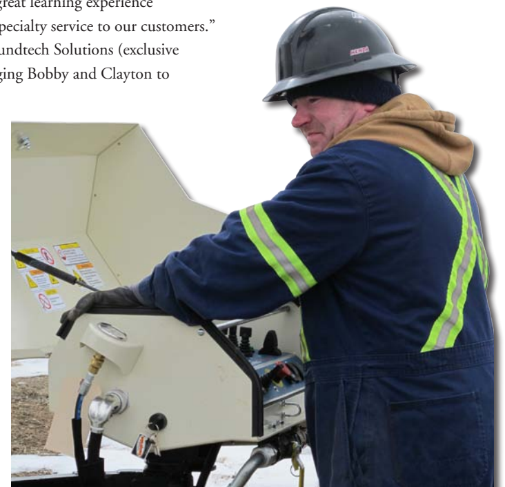
Clayton Duralia with Omega Environmental Drilling in Vancouver, learns the controls of the Geoprobe® 8140LS Rotary Sonic.
