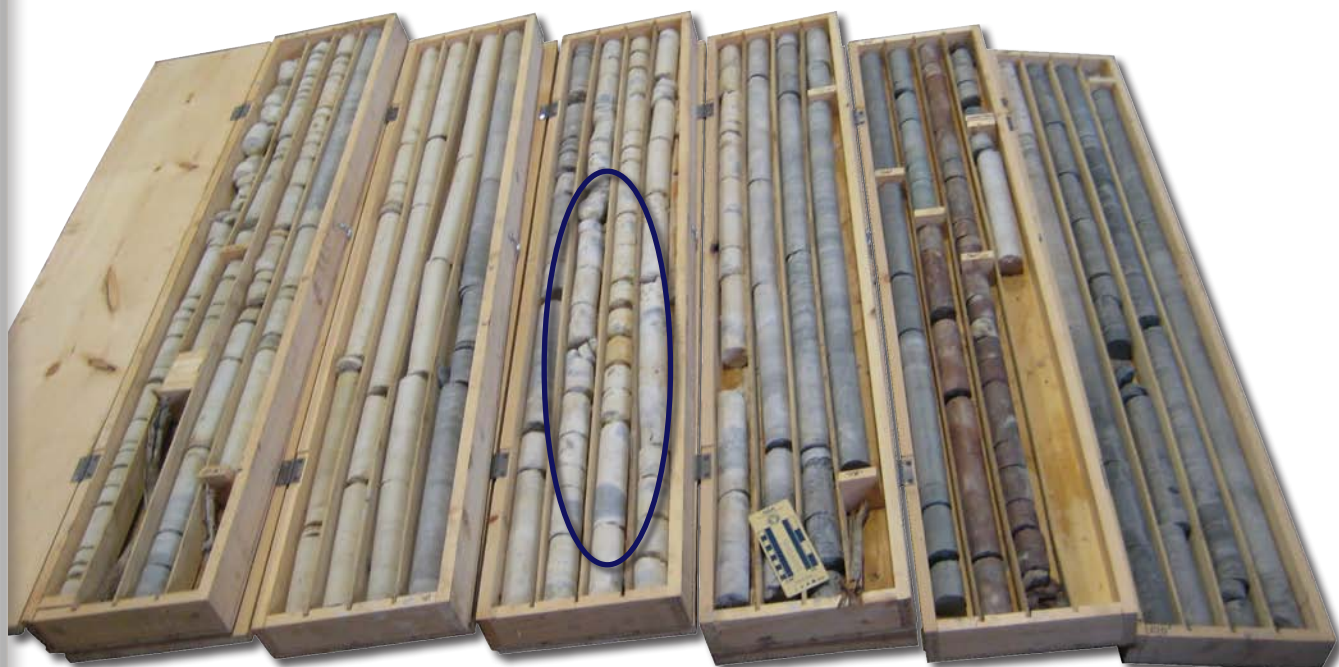
These core boxes hold the top 115 feet of rock cores taken at the Geoprobe® test site in Marion County, KS. The top of the first core is shown upper left. The blue oval shows where gray chert nodules are present in some of the buff colored limestone. The last two boxes on the right contain dark, greenish gray-to-red shale. The upper 40-ft. of the formation is comparable to the exposed rock face shown on next page.
