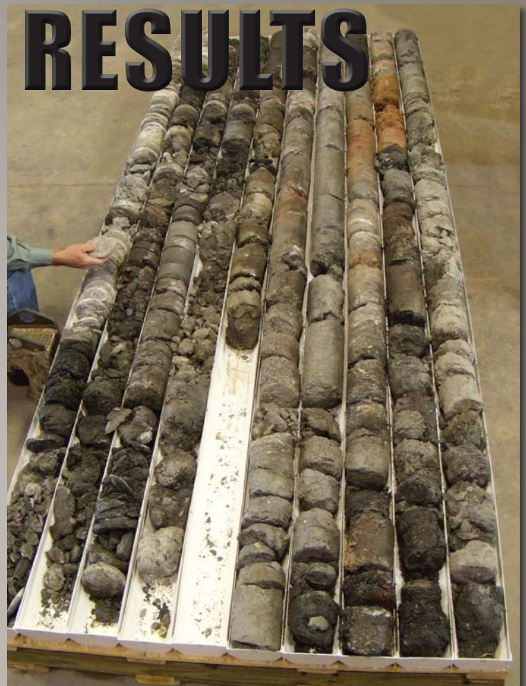
Geoprobe® Tooling Engineers collected 200 ft. (61 m) of cores in the backyard using a Geoprobe® 8140LS Rotary Sonic and SDT60 (sonic dual tube 6 in. OD) tooling. Each of the recovered core samples was approximately 4.3 in. (109 mm) OD and 10 ft. (3 m) in length. This photo shows the bottom 100 ft. (30 m) of the 200 ft. boring. The top of the core segment is at the lower right, and the final 10 ft. segment begins at the upper left.
