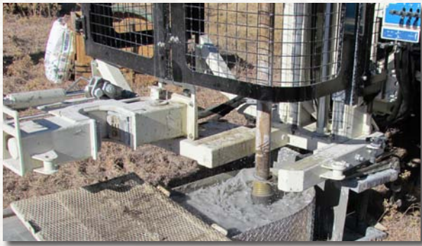
New 7-in. Single Rod Breakout
