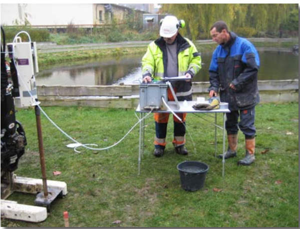
Robert Berlowicz (left) and Thomas Layborn, both with NIRAS, collect groundwater samples at location SK04. The SP16 Groundwater Sampler was installed with a 30 cm (1 ft.) screen interval at increasing depths for profiling water quality. The Mechanical Bladder Pump and 12V actuator were used for pre-sample purging and sampling of X-VOCs. Robert records water quality parameters as Thomas prepares to collect a sample. The former machining/manufacturing building is in the background.
