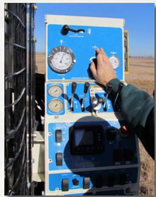
New Head Feed Pressure Control module for the 7822DT Control Panel
