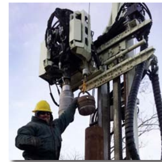
Bryan Marshall, 8140LS Operator, gets up close with the 10 in. x 10 ft. sonic casing.
