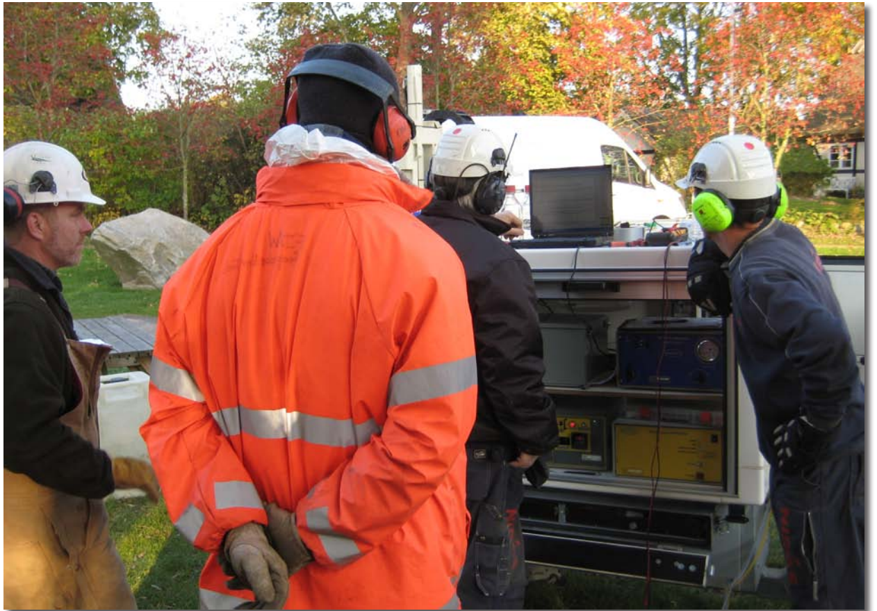
(left to right) Dan Pipp, Geoprobe® Chemist; Fabian Deweydt, Geoprobe® Environmental Technologies, (GET) Belgium; Peter Stig Thomsen, NIRAS, MIP Operator; and Thomas Layborn, NIRAS, MIP/Geoprobe® Machine Operator. Conducting response tests and reference tests on the MiHpt probe before a log is started. NIRAS has a specially designed MIP 'wagon' to move the MiHpt instrumentation around the site.
