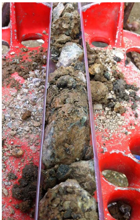
The 54LT and MC5 soil sampler had no problems with the large, gravelly materials encountered at the Cape Newenham drilling location.
