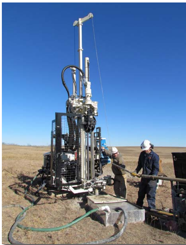
Joel Christy (left) and Nathan Peters, members of the Geoprobe® Engineering Team, core to 150 feet using the new 7822DT rig and industry standard NQ wireline diamond core drilling tools.
