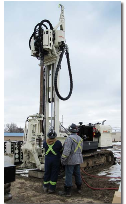
Clayton Duralia (left) and Bobby Tura, with Omega Environmental Drilling in Vancouver, learn the art of sonic drilling during their two-day training.
