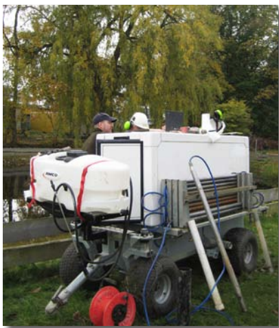
NIRAS uses a mobile Direct Image® logging trailer to transport their DI equipment and tooling to various sites. The trailer also protects the instrumentation inside during the process logging.
