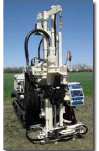
(right) A very visible E-stop (red) with cable is located next to the rig operator's work space, accessible to trip for any emergency during operation.
