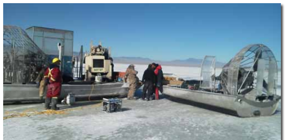
(left) Ryan Roodbol (left), Darin Bromley, and Dusty Swant use the 7730DT to collect continuous soil cores from the lake bed while sampling through shallow depths of water. The rig is carried on a marsh airboat for the project while core samples were taken and temporary piezometers were installed at over 400 hole locations. (above) Field team members: (l to r) Ryan Roodbol (seated), Dusty Swank, Clay Smith, Darin Bromley, Verl King and Trevor Pulham. Two marsh airboats were used to transport the 66DT and 7730DT across the lake bed. While working on the water, the field team encountered wind, rain, and snow with temperatures ranging between 50 degrees to below freezing.
