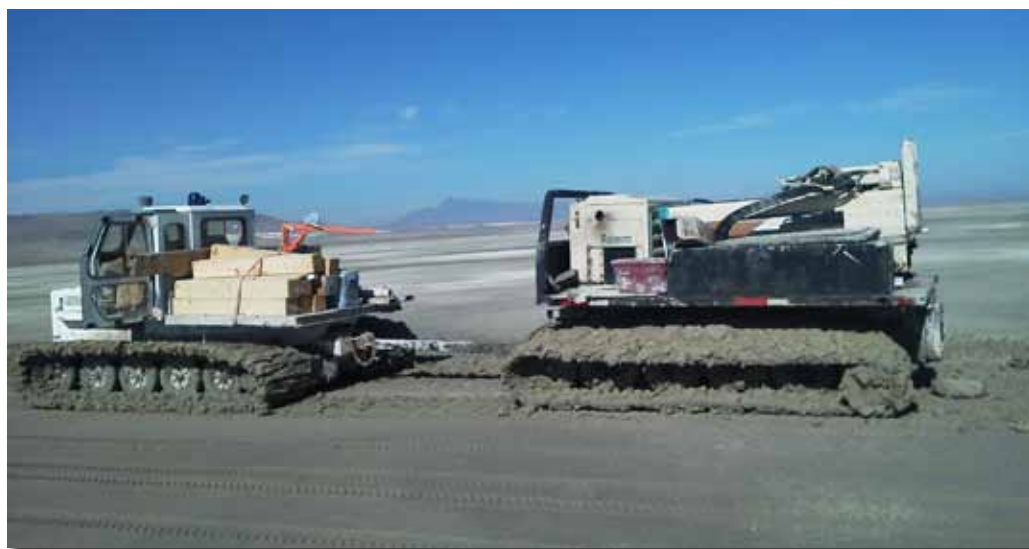
Direct Push Services removed their 6600/BP power unit (above right) from its truck carrier vehicle and mounted it on a heavy-duty Sno-Cat® trailer which was pulled behind a heavy-duty diesel Sno-Cat® with 5-ft. wide tracks (above left).
