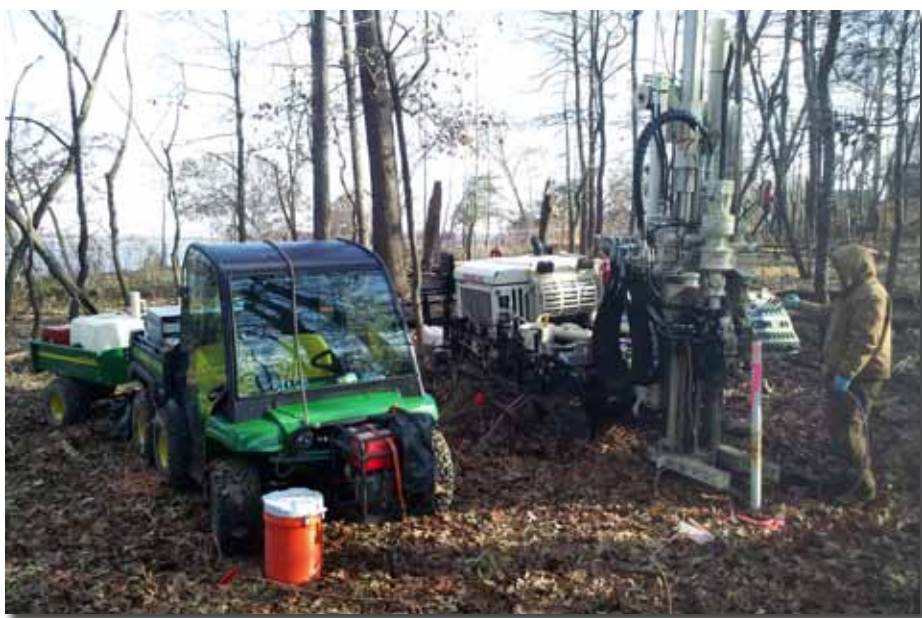
S2C2 used their 7822DT and 6620DT (not pictured) supported by a six-wheel-drive Gator ® for the direct sensing project in Maryland.
