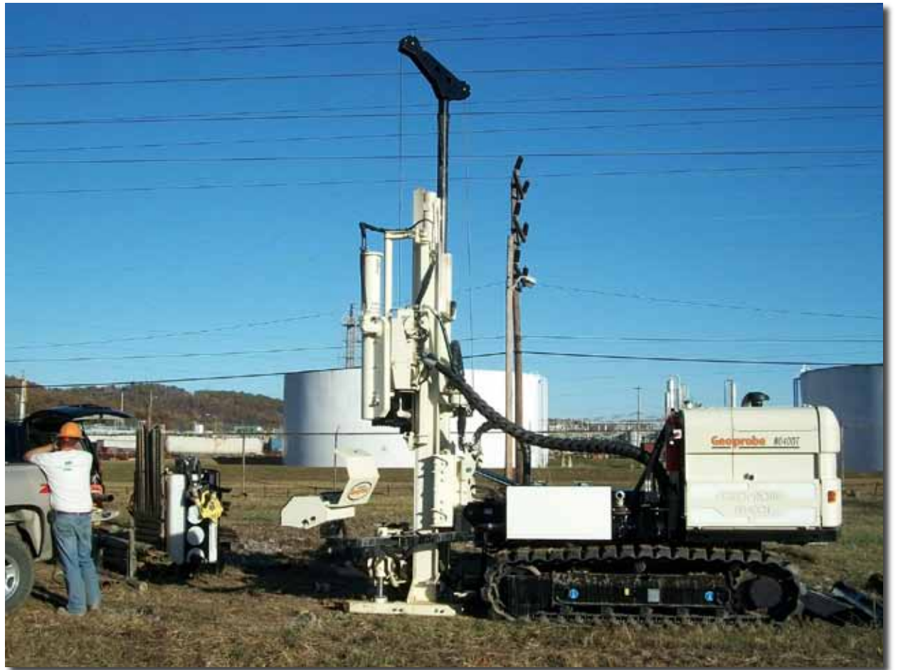
The EnviroProbe Integrated Solutions field team uses the 8040DT with DT45 and MCS tooling to collect soil cores at an industrial site. Up to three discrete groundwater samples were collected per location using the SP16 Groundwater Sampler.
