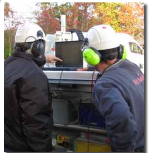
Peter Thompsen (left) and Thomas Layborn of NIRAS S/A in Allerød, Denmark, review the MIP detector results and HPT pressure log onscreen as the MiHpt probe is advanced. Having the HPT pressure log along with the detector results is useful in understanding how the lithology controls contaminant migration.
