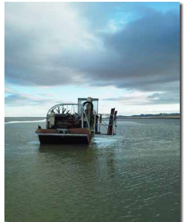
A marsh airboat was used to maneuver the 66DT in areas of the lake that still contained water; typically 3 in. to 2 ft. in depth. The field team collected soil cores from the lake bed sediment and installed small diameter temporary piezometers throughout the 30-mile radius of the lake.
