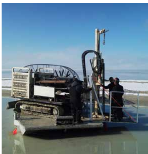
Direct Push Services removed their 6600/BP power unit (above right) from its truck carrier vehicle and mounted it on a heavy-duty Sno-Cat® trailer which was pulled behind a heavy-duty diesel Sno-Cat® with 5-ft. wide tracks (above left).
