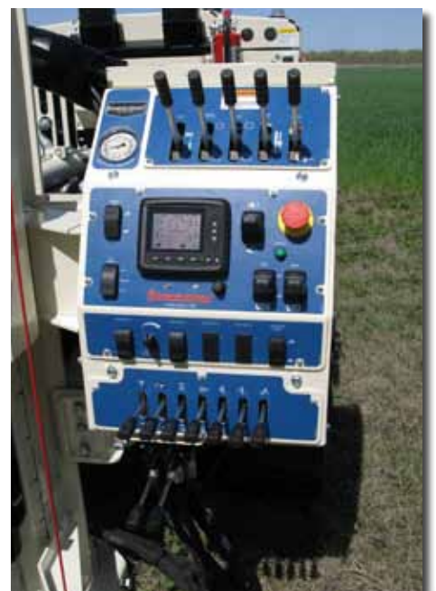
Driven by a desire to conform to the new 2012 CE safety standards, the new control panel design for the 7822DT with new Operator Interface has a digital display screen with multi-function output and advanced warning displays.
