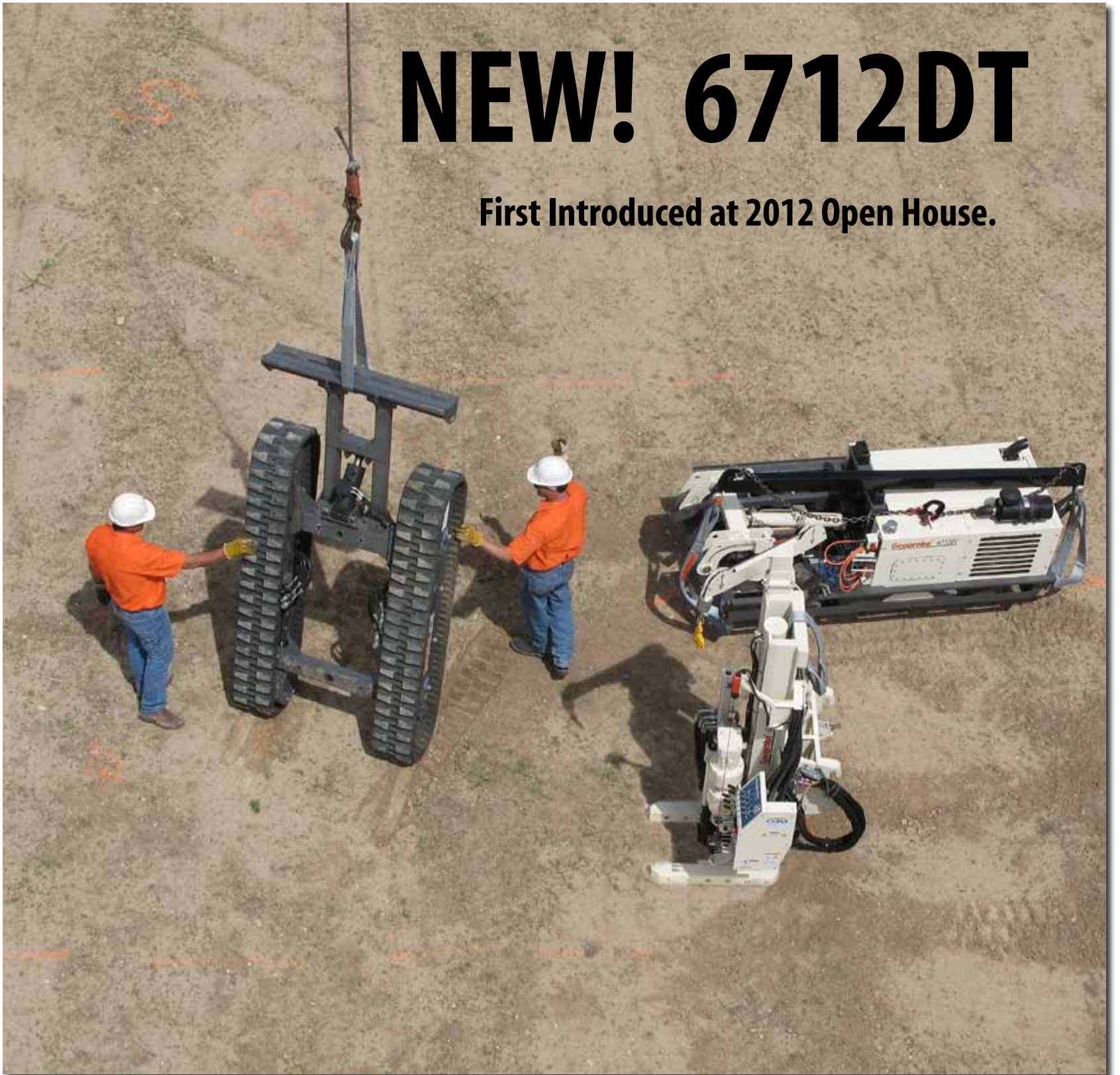
The new Geoprobe® 6712DT separates into three sections for easy transport. Mark Abker (left) and John Frost, both Geoprobe® Engineers, reassembled the rig at Open House in 10 minutes.
