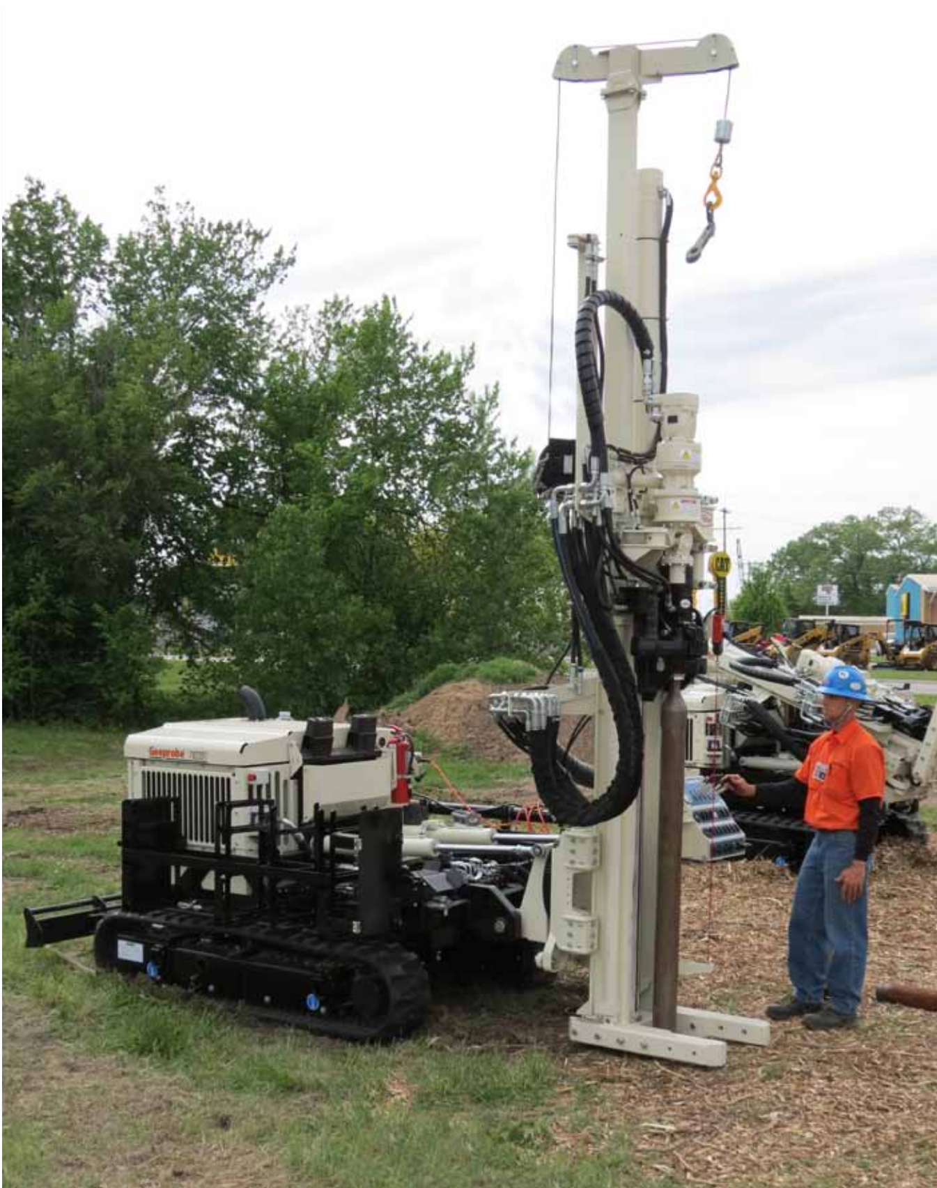
Lee Shaw, Geoprobe® Customer Service, demonstrates the use of DT 325 tooling with the 7822DT at the 2012 Open House in April. The 7822DT is fast becoming known as a real work horse in the field. Geoprobe® customer service staff almost daily receives feedback from the field that operators continue to discover new capabilities and uses for the rig including air rotary and wet rotary.
