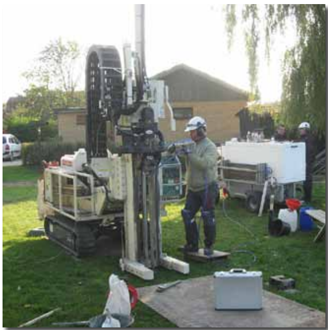
Martin Eklund of NIRAS S/A in Denmark advances the MiHpt probe at one of the first locations logged at the X-VOC contaminated area in Skuldelev, Denmark, in October 2011. In the background, Thomas Layborn and Peter Thompsen observe the log results onscreen at the NIRAS MIP Wagon.
