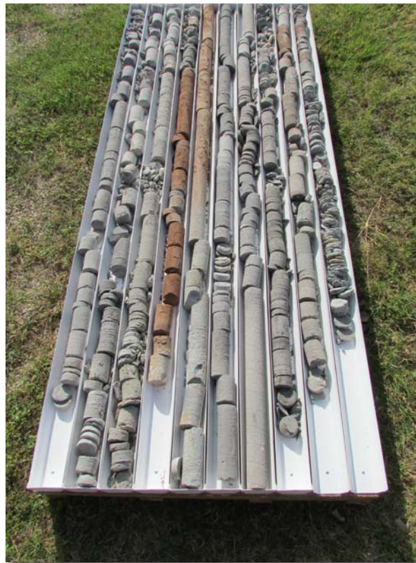
Soil cores taken with the 10-ft. SDT45 system. Cores were collected from 200 to 300 feet during Geoprobe® R&D testing.
