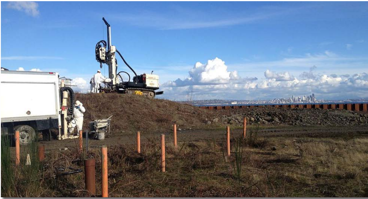
Eric Nuchims, Chemist with Ecology and Environment in Seattle, WA, spent two weeks on Bainbridge Island, WA, using a 6600 (foreground) at an environmental investigation. It was his first time operating a rig alongside a master operator, Alan Jensen. An 8140 rotary sonic is shown working atop the hill. Downtown Seattle, WA, is in the background.
