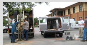
FL DEP personnel use their 6600 to advance the HPT-GW sampler onsite in Pensacola, FL.
