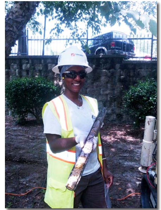
Pamela Oree, Engineer with Schnabel Engineering, holds a split spoon soil sample collected from 30 ft. below ground surface.
