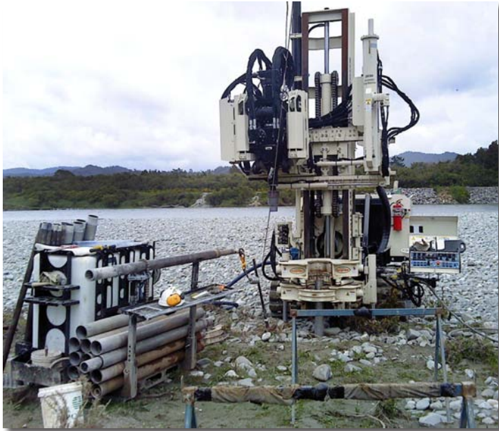
Iain Haycock, Manager for McMillan Drilling Services in Canterbury, New Zealand, used their 8140LC rotary sonic and DT45 to retrieve samples of mostly cobble-sized Greywacke ("hard, to say the least!") on the west coast of the south island of New Zealand. The filled liners contained vesicular Basalt rock. The field team was impressed with the recovery and lack of drilling-induced fractures.
