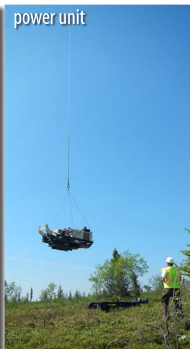
(above left) First the drill mast section of the 6712DT is mobilized to the site via helicopter. (above center) Then the tracks are lowered to the site. (above right) And finally, using a helicopter long-line system, the power unit of the 6712DT joins the other two sections on the ground. (below right) The power unit attaches to the tracks by tightening four bolts and connecting a series of quick connect hydraulic fittings. The drill mast connects to the power unit with two bolts and another series of quick connects. Assembly takes approximately 15 minutes, then the rig is ready to roll.
