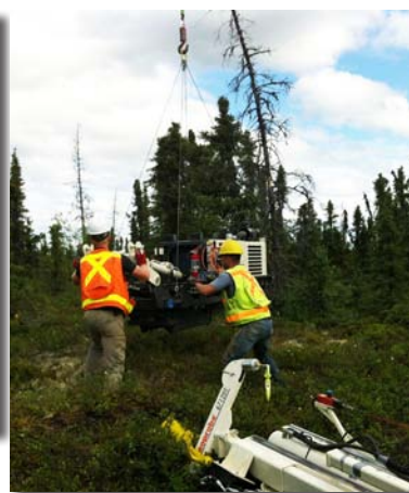
(above left) First the drill mast section of the 6712DT is mobilized to the site via helicopter. (above center) Then the tracks are lowered to the site. (above right) And finally, using a helicopter long-line system, the power unit of the 6712DT joins the other two sections on the ground. (below right) The power unit attaches to the tracks by tightening four bolts and connecting a series of quick connect hydraulic fittings. The drill mast connects to the power unit with two bolts and another series of quick connects. Assembly takes approximately 15 minutes, then the rig is ready to roll.
