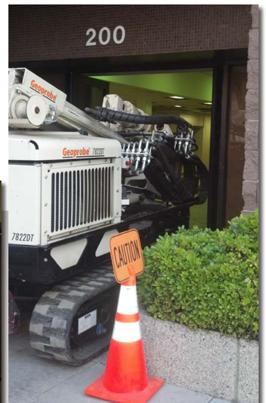
Glenn Reiss, Owner/Geologist with Vapor Tech Services in Hayward, CA, guides a 7822DT through a building entrance. Seventeen remediation wells were installed inside the building.
