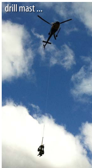
(above left) First the drill mast section of the 6712DT is mobilized to the site via helicopter. (above center) Then the tracks are lowered to the site. (above right) And finally, using a helicopter long-line system, the power unit of the 6712DT joins the other two sections on the ground. (below right) The power unit attaches to the tracks by tightening four bolts and connecting a series of quick connect hydraulic fittings. The drill mast connects to the power unit with two bolts and another series of quick connects. Assembly takes approximately 15 minutes, then the rig is ready to roll.
