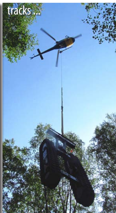
(above left) First the drill mast section of the 6712DT is mobilized to the site via helicopter. (above center) Then the tracks are lowered to the site. (above right) And finally, using a helicopter long-line system, the power unit of the 6712DT joins the other two sections on the ground. (below right) The power unit attaches to the tracks by tightening four bolts and connecting a series of quick connect hydraulic fittings. The drill mast connects to the power unit with two bolts and another series of quick connects. Assembly takes approximately 15 minutes, then the rig is ready to roll.
