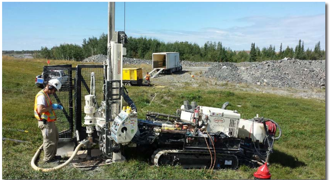
Scott Reid, Driller with Strata Drilling, checks his notes. This 7822DT is equipped with a rotational safety cage that remains closed during drilling operations.
