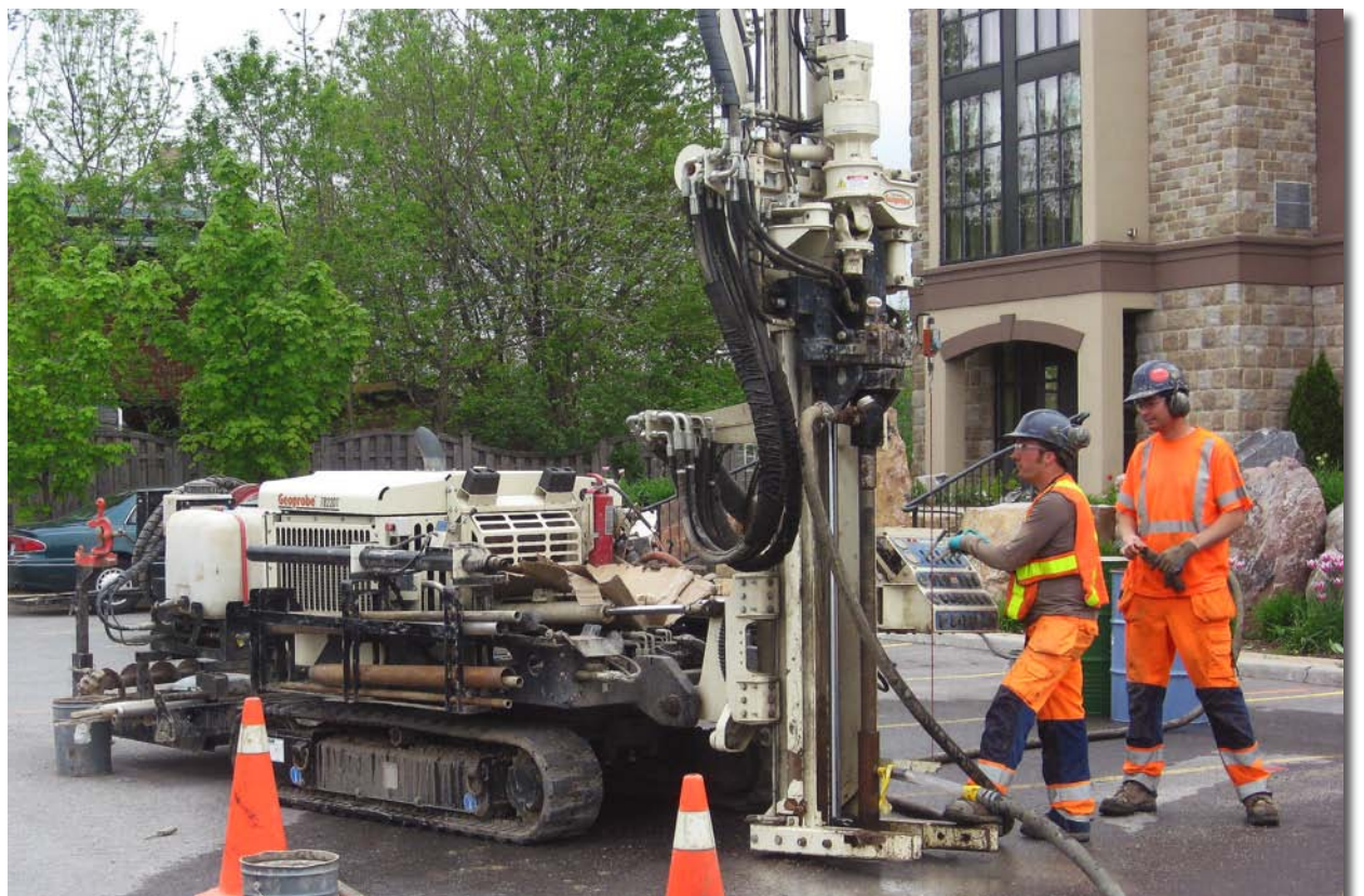
Strata Drilling personnel Phil Halladay, Driller, operates the 7822DT with Rob Parsons on an environmental site in Ottawa.
