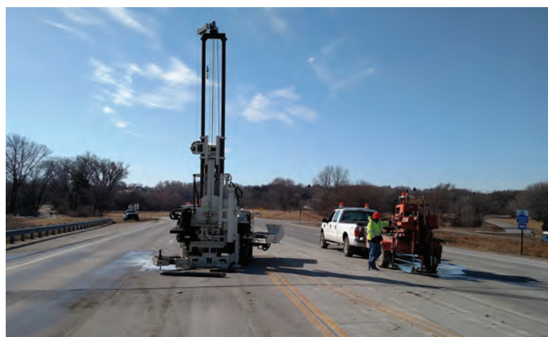
Left: The Nebraska Department of Transportation performs a forensic investigation in the approach fill at the Platte River Bridge south of Fremont, NE. Direct push sampling with the 3230DT allowed NDOT to immediately review samples to see if frozen soil or ice lenses were present and could have caused the pavement to heave and crack.
