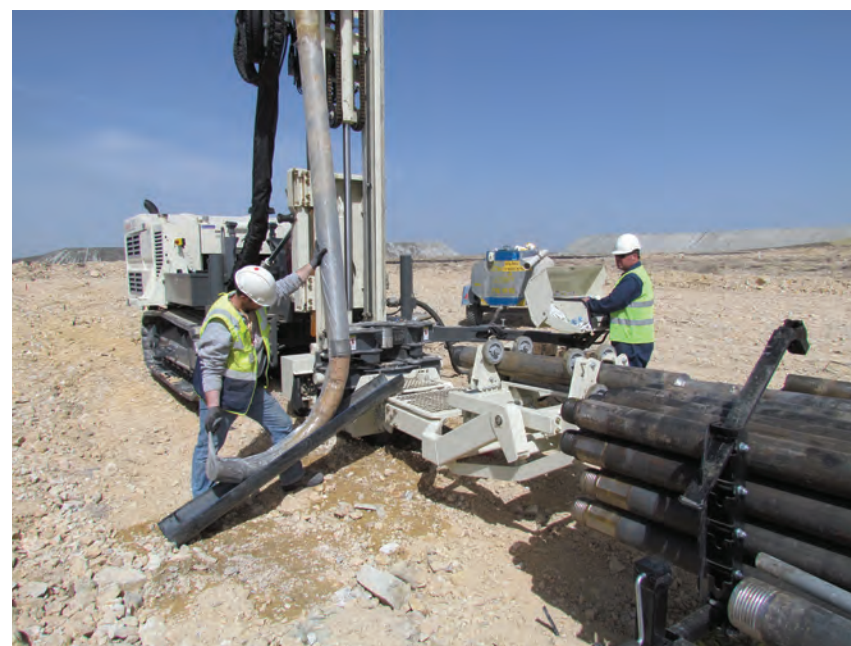
Top and Bottom: Geoprobe® Engineer Joel Christy leads sonic training for the drill crew at the Kisladag Gold Mine in Turkey. The training used 6x8 in. coring through crushed rock of a heap leach pad using Geoprobe® 4.5 in. Heavy Duty (HD) rods as the working rod to drive the 6 in. barrel.
