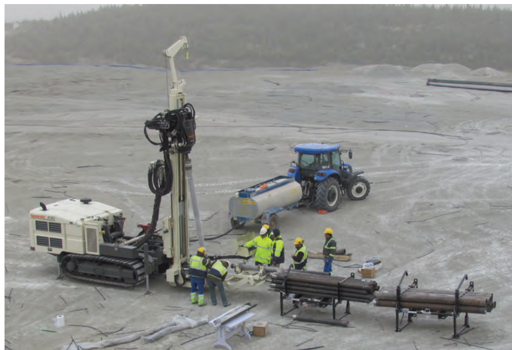
Top and Bottom: Geoprobe® Engineer Joel Christy leads sonic training for the drill crew at the Kisladag Gold Mine in Turkey. The training used 6x8 in. coring through crushed rock of a heap leach pad using Geoprobe® 4.5 in. Heavy Duty (HD) rods as the working rod to drive the 6 in. barrel.
