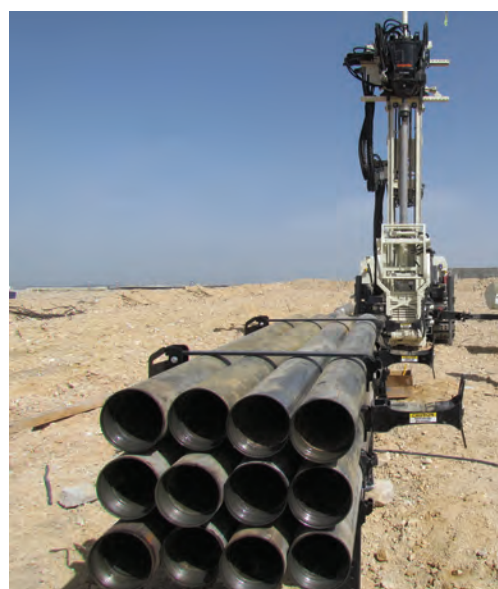
The drill crew at the Kisladag Gold Mine in Turkey utilize two Geoprobe® Indexing Racks to position the Geoprobe® 4.5 in. Heavy Duty (HD) sonic rods into the grippers of the rig-based rod handler on the 8150LS rotary sonic machine. Pictured are the 4.5 in. HD sonic rods and indexing racks at the gold mine in Turkey.
