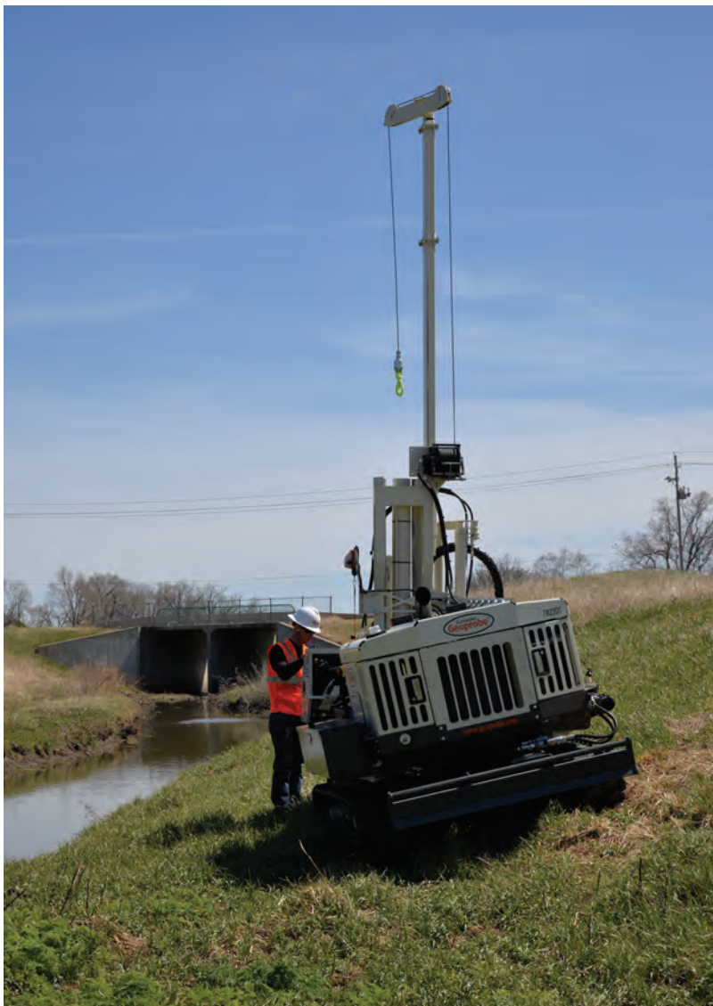
The Geoprobe® 7822DT V3 is easy to mobilize on unlevel terrain. The oscillation feature allows the rig to be on a slope at an angle while the drill mast is vertical.
