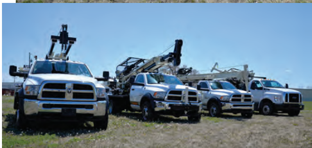
Here is an example of Geoprobe® and DRILLMAX® machines that can be mobilized to job sites without the use of a CDL. In some cases, DOT weight restrictions require project tooling and supplies to be carried on a support vehicle.
