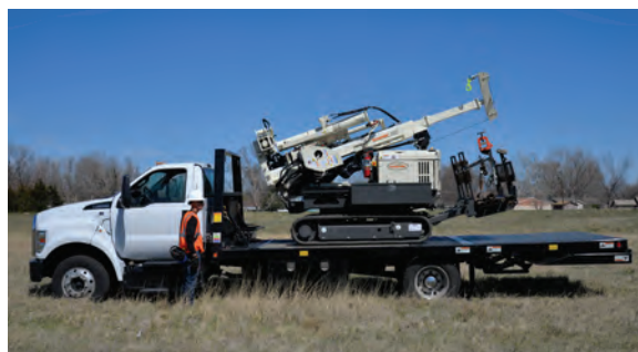
NO CDL REQUIRED: Loading and transporting a 7822DT is easy using this F650 transport truck with EZ12 bed.
