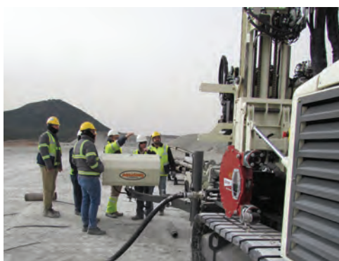
Top and Bottom: Geoprobe® Engineer Joel Christy leads sonic training for the drill crew at the Kisladag Gold Mine in Turkey. The training used 6x8 in. coring through crushed rock of a heap leach pad using Geoprobe® 4.5 in. Heavy Duty (HD) rods as the working rod to drive the 6 in. barrel.
