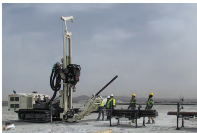
The drill crew at the Kisladag Gold Mine in Turkey operate the Geoprobe® 8150LS Sonic rig and Geoprobe® 4.5 Heavy Duty (HD) sonic drill rods.
