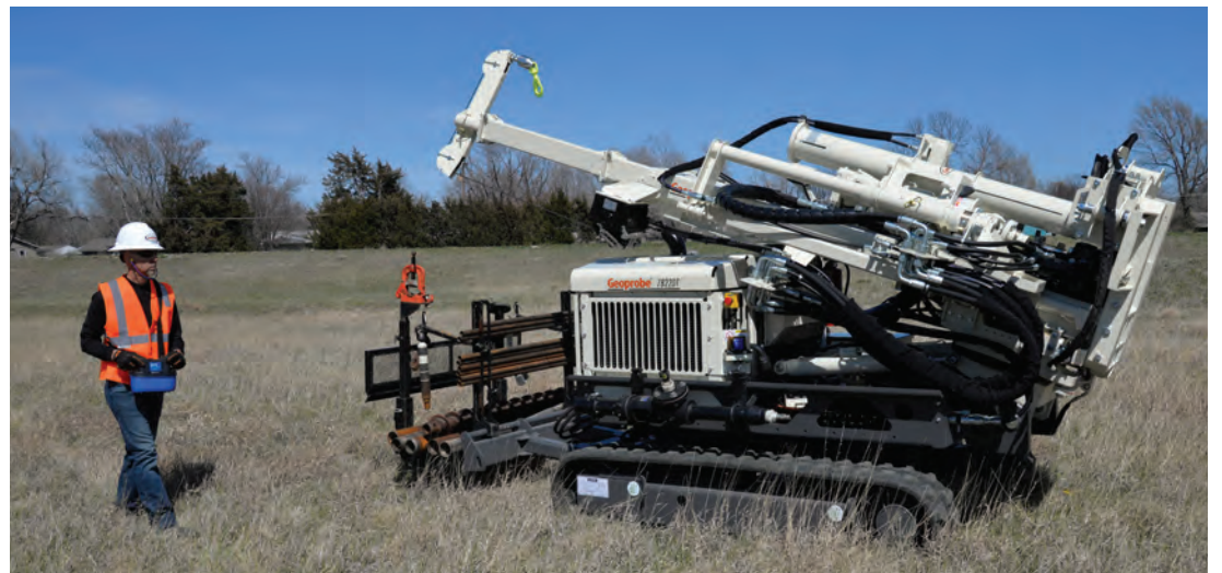
The Geoprobe® 7822DT V3 is easy to mobilize on unlevel terrain. The oscillation feature allows the rig to be on a slope at an angle while the drill mast is vertical.
