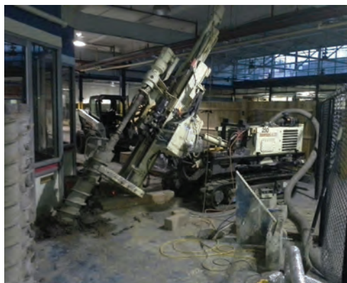
MiHpt Operator Matt Padgett uses the 6712DT in an urban setting in North Carolina to collect MiHpt.
