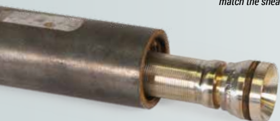
Geoprobe® SP19 with top of screen larger to match the sheath
