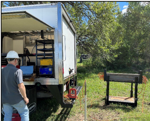
Figure 6: Probe rods are prestrung with the HPT trunkline and may be stored and transported on a Geoprobe® drop rack. In this setup the water tank, generator and instrumentation may be loaded in a vehicle for easy transportation on site.
