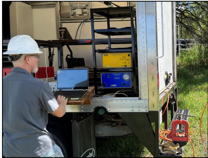
Figure 7: The HPT flow controller (bottom) draws water from the tank (upper left) and regulates flow to the probe. The FI 6000 Field Instrument (top) supplies conditioned current for the EC measurement, receives analog signal from the HPT probe and provides digital output to a lap top computer (left).
