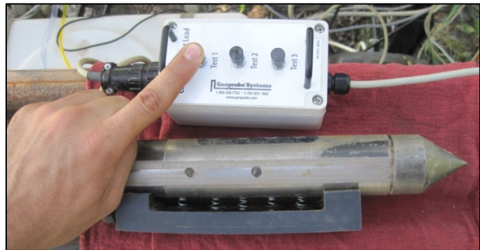
Figure 8: As part of the field QA testing the EC probe is setup in the test jig (bottom) and the EC test load (top) is used to verify the performance of the EC array before each log is run. The QA results are saved in the information file (Appendix I).
