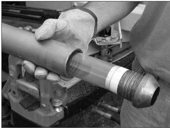
Figure 4.8. Slide whole assembly into either end of the sample tube.
