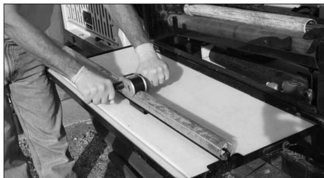
Figure 4.33. MC Liner Cutter makes two longitudinal cuts in PVC Liners.
