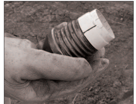
Figure 4.1. The spacer ring fits securely onto the MC5 Cutting Shoe.
