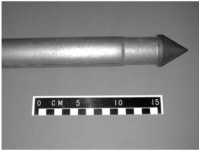
Figure 5. (a) Shielded screen tool with screen shroud in place; (b) Shielded screen tool after screen shroud has been pulled back
