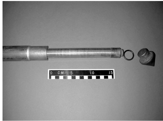
(well point with O-ring always left in formation; rubber plug at bottom of screen can be knocked out for retraction grouting).
