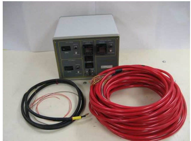
Figure 6: Heated Trunkline Controller, 8 ft. Transfer Line, 150 ft. Heated Trunkline
