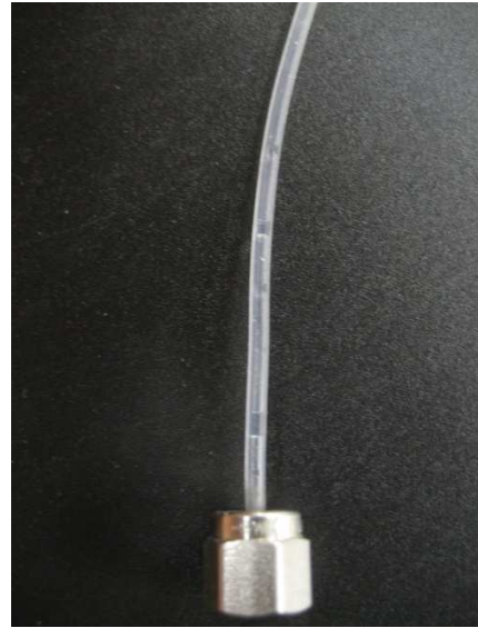
Figure 5: Condensation in trunkline
