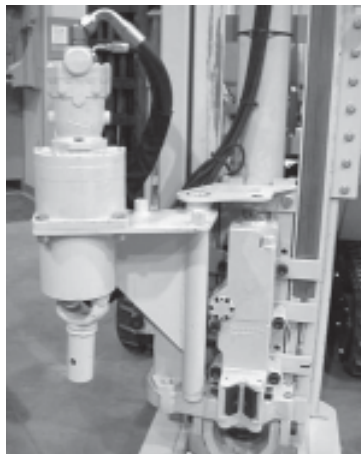
Figure 1. Augerhead rotated to access hammer.
