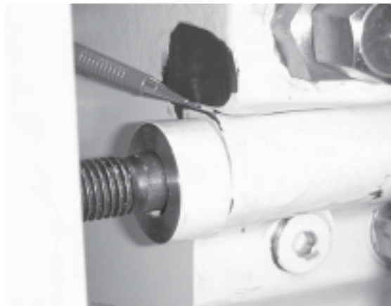
Figure 18. Rear view of hammer showing upper socket head cap screw as taken from side opposite control panel. Pencil shows junction between upper and middle hammer housings. Spacer must not contact upper housing (above pencil).
