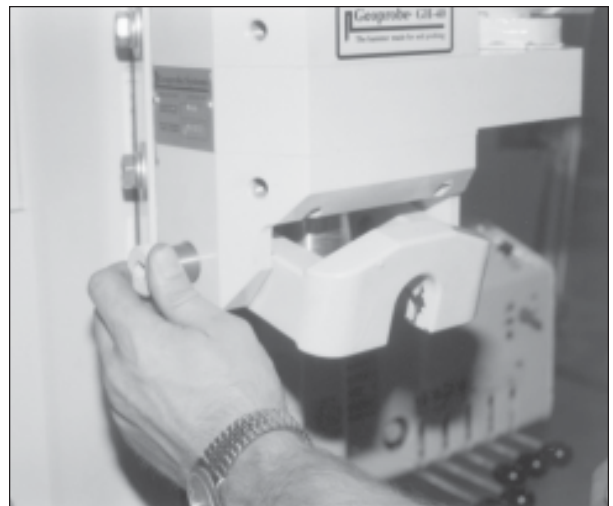
Fig. 22.12. Install shoulder bolt through the latch extension into the hammer latch.
