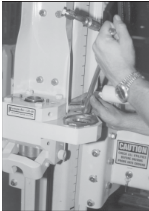
Fig. 18.22B. Reinstall lower mounting bolts.
