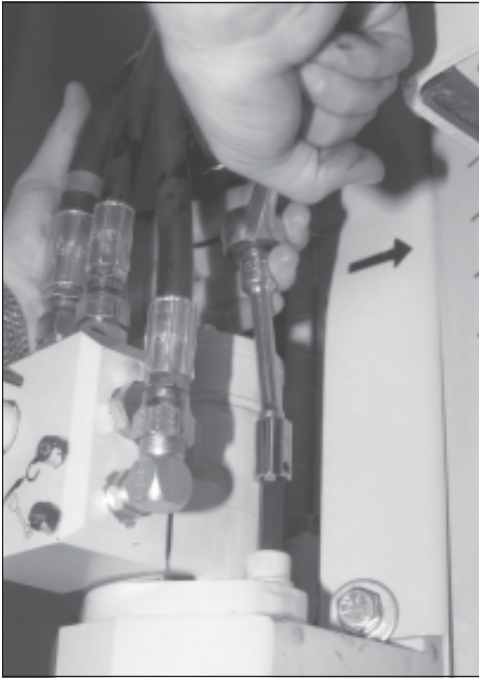
Fig. 17.5. Remove socket head cap screws from hydraulic motor mounting holes.
