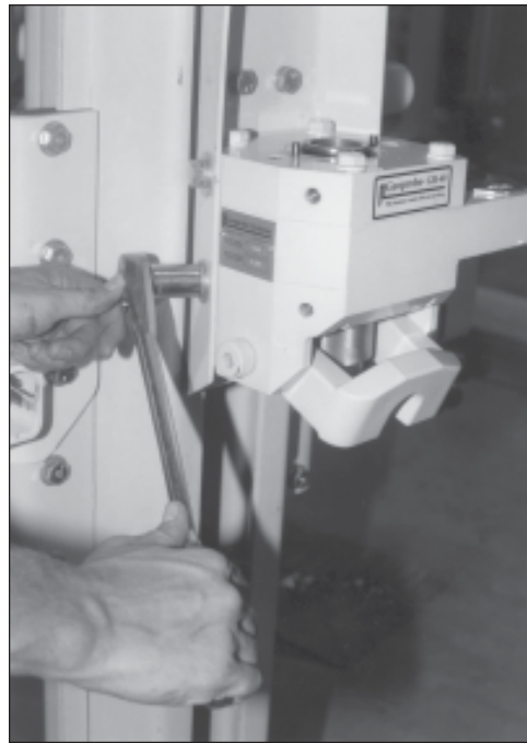
Fig. 18.22A. Reinstall lower mounting bolts.
