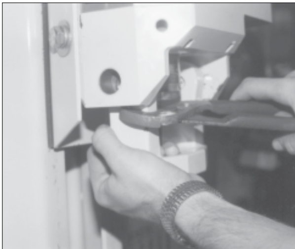
Fig. 22.9. Push latch towards bottom plate while holding detent ball inside of latch.
