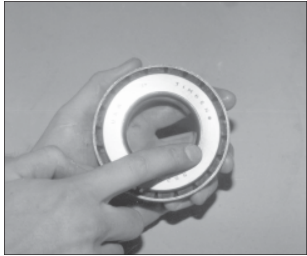
Fig. 18.5B. Make sure inner race surfaces are free of grease.
