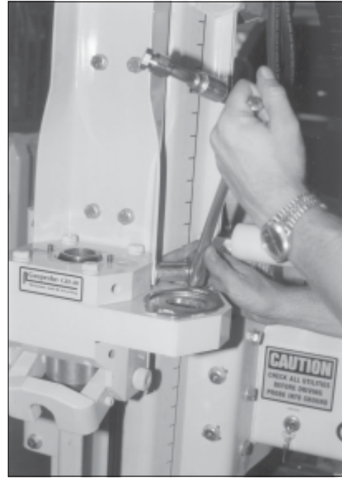
Fig. 17.9B. Remove lower mounting bolts.
