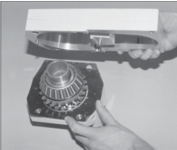
Fig. 17.15. Lift gear drive box off bottom plate.
