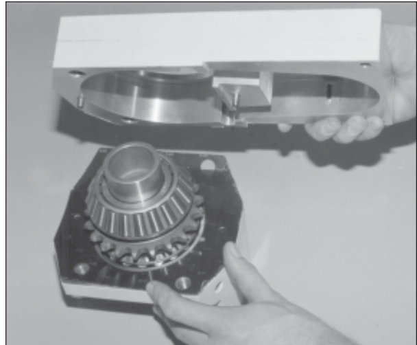
Fig. 18.13. Place gear drive box on bottom plate and shim making sure shim does not wrinkle.
