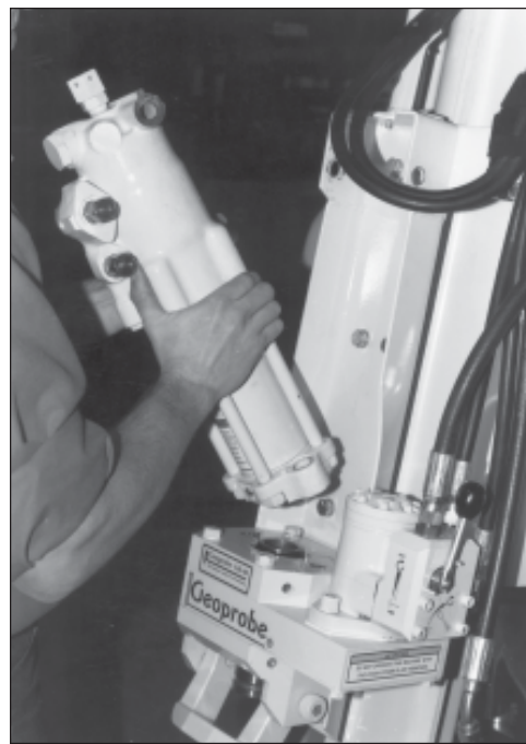
Fig. 18.25. Reinstall hammer member.
