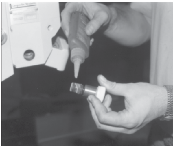
Fig. 22.11. Apply Loctite Removable Threadlocker on shoulder bolt threads.
