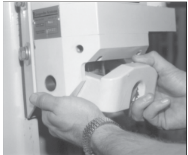
Fig. 22.10. Pivot latch upward until detent ball snaps in place.
