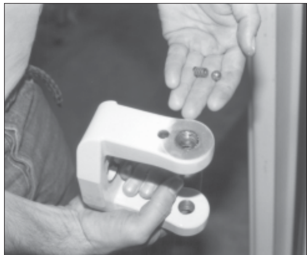
Fig. 21.5. Locate ball bearing and spring and set aside.
