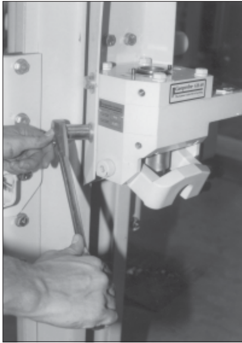
Fig. 17.9A. Remove lower mounting bolts.
