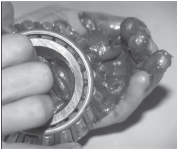
Fig. 18.3. Pack tapered roller bearings with wheel bearing grease.
