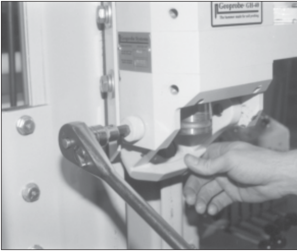
Fig. 22.13. Tighten both socket head shoulder bolts.
