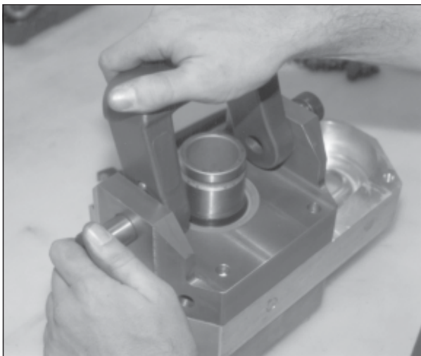
Fig. 20.11. Insert left-side shoulder bolt just far enough to align hammer latch indenture with latch extension.
