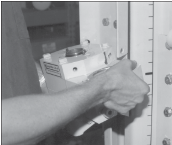
Fig. 17.10A. Lift rotation member out of hammer cradle.
