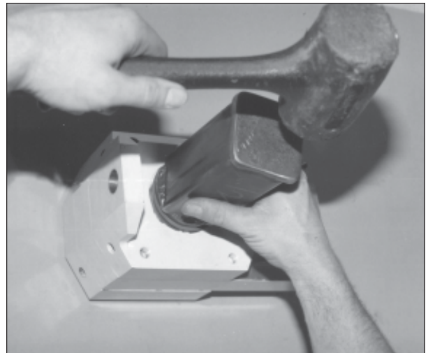
Fig. 18.19A. Seal is tapped into place using a seal installer. (Option 1)
