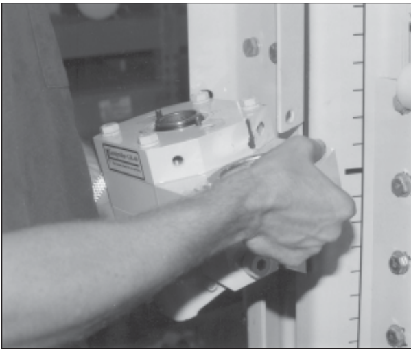
Fig. 18.21. Reinstall GH-40 rotation member in hammer cradle.
