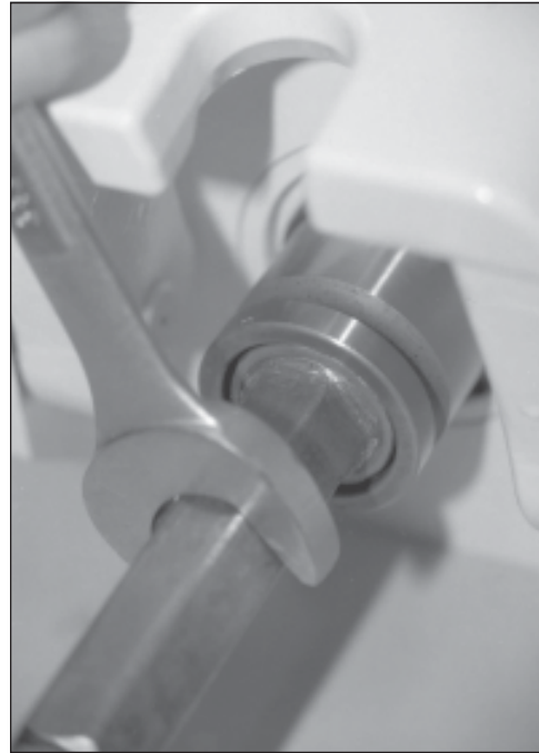
Fig. 18.17. Install drill steel, if necessary, to check hex drive gear for proper rotation.
