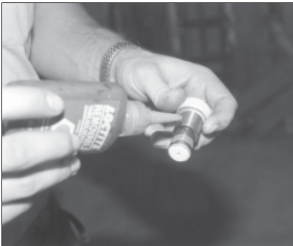
Fig. 22.3. Apply Loctite Removable Threadlocker to hammer latch shoulder bolt.
