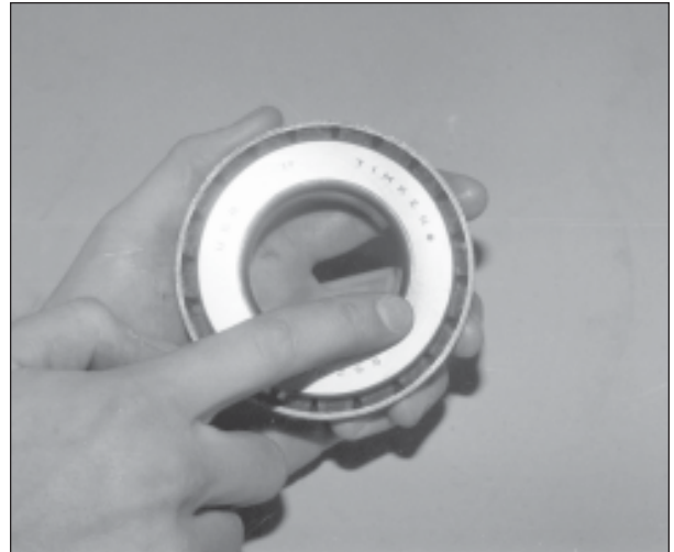
Fig. 18.10A. Inner bearing race mating surface should be free of grease.
