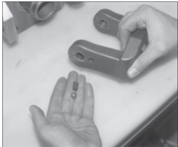
Fig. 19.4. Locate detent ball and spring and set aside.
