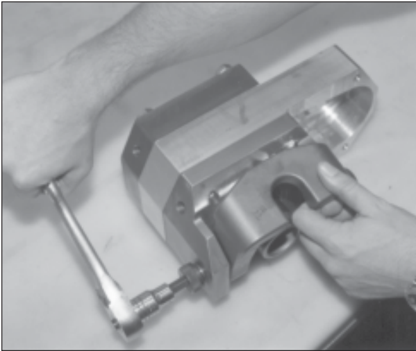
Fig. 19.1. Loosen shoulder bolts and latch assembly from bottom plate.
