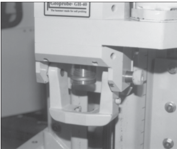
Fig. 22.5. Screw bolt in bottom plate just enough to hold latch.
