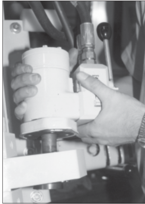
Fig. 17.6. Lift hydraulic motor off gear drive box.
