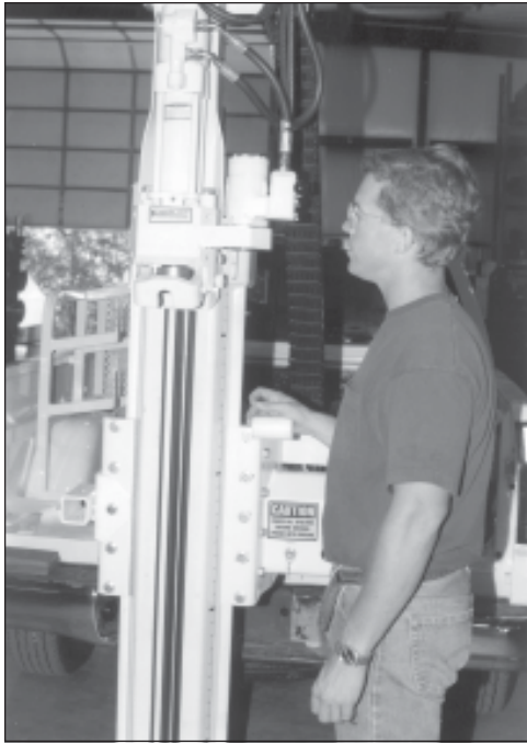
Fig. 21.1. Lift hammer to top of stroke.
