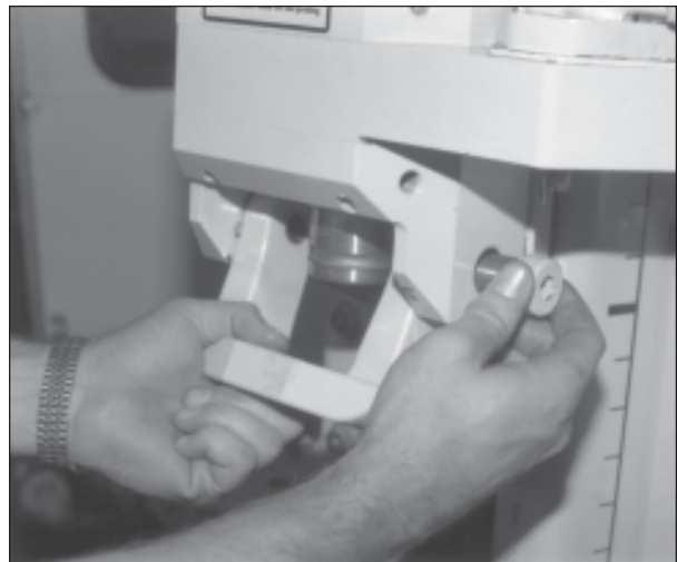
Fig. 22.4. Install shoulder bolt on the side of latch opposite detent ball indentation.
